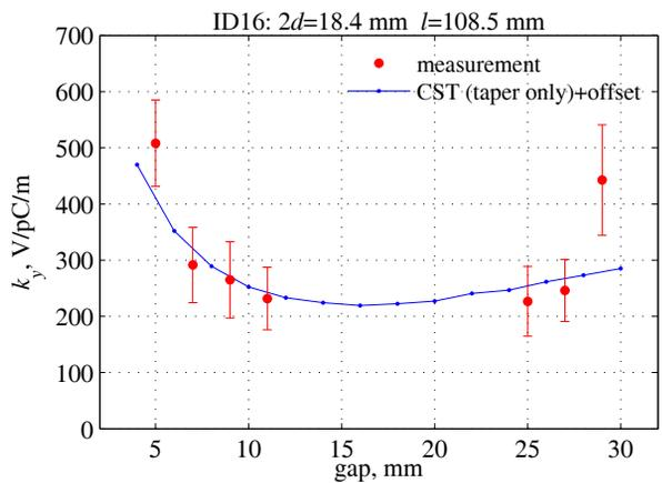
Figure 6: Vertical kick factor vs ID gap.
