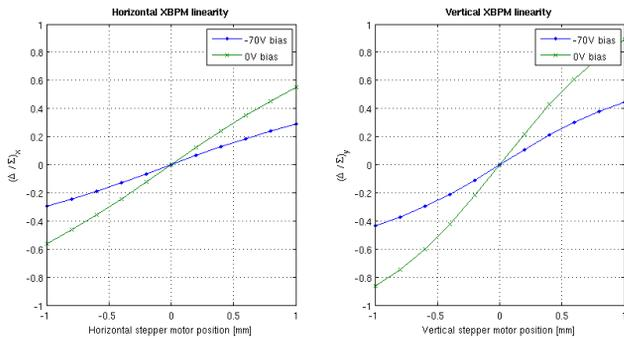
Figure 9: The linearity of the XBPM measurements for horizontal and vertical stepper motor displacements.
