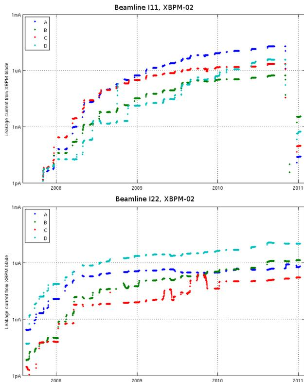
Figure 3: Blade currents (blade A, B, C, D) for XBPM-02 on the I11 beamline, top, and XBPM-02 on the I22 beamline, bottom. These two XBPMs exhibited the largest leakage currents seen at DLS. In November 2010 the ceramic insulation was replaced in the I11 XBPM, reducing, but not eliminating, the leakage current.
