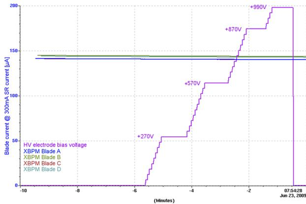
Figure 6: Results from I16, XBPM-01. As the HV electrode was ramped up to +1000V under nominal conditions (300 mA stored beam current, ID at 7.0 mm gap) the XBPM blade response was recorded. Negligible difference was seen to either the overall currents, or the signal/noise ratio.
