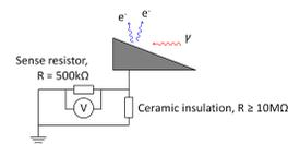
Figure 10: A sense resistor can be substituted for the ammeter, so long as the  $I_{sense} \gg I_{leakage}$ .
