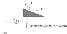
Figure 1: An illustration outlining the principal of operation behind the XBPMS. The ceramic insulation that is used to hold the XBPMS blades in place, and to electrically isolate them from the rest of the XBPMS chamber, is indicated by the resistor.
