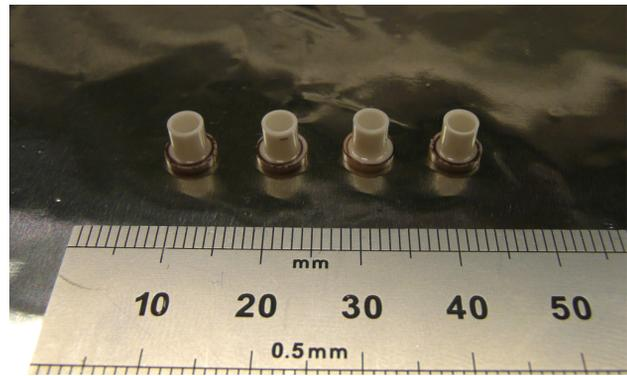
Figure 4: The ceramic sleeves that electrically isolate the XBPM blades from the XBPM vessel. Dark-coloured deposits are visible on the white ceramic surface.
