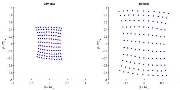
Figure 8: Results from a 2D stepper motor scan of the I24 XBPM-01 with, and without bias. The recorded  $\Delta/\Sigma$  position measurements are shown, with points evenly spaced: each represents a 200  $\mu\text{m}$  stepper motor movement.
