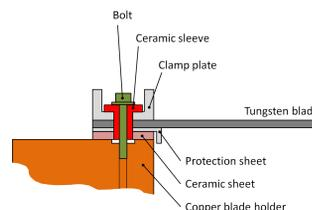
Figure 2: A schematic showing the insulation, and how the tungsten blade is fixed to the copper blade holder.
