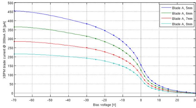
Figure 5: Measured XBPM blade response for varying ID gaps on I11. As one increases the bias voltage from 0 V to -70 V the signal increases, improving signal/noise.
