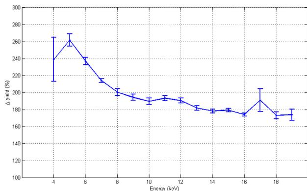
Figure 7: Experimental results showing the % increase in XBPM signal that a -70 V bias causes (compared to no bias), for various X-ray energies. The -70 V bias has a tendency to preferentially select soft X-rays. These results were obtained using dedicated beam time on the B16 Test Beamline at Diamond.
