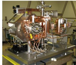
Figure 4: LCLS photocathode gun with solenoid, water feeds and RF waveguide.
