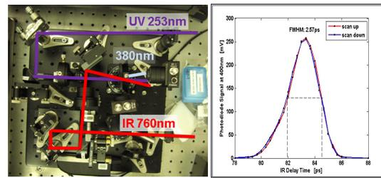
Figure 3: (a) Plan view image of UV/IR cross-correlator and (b) typical cross-correlation scan.
