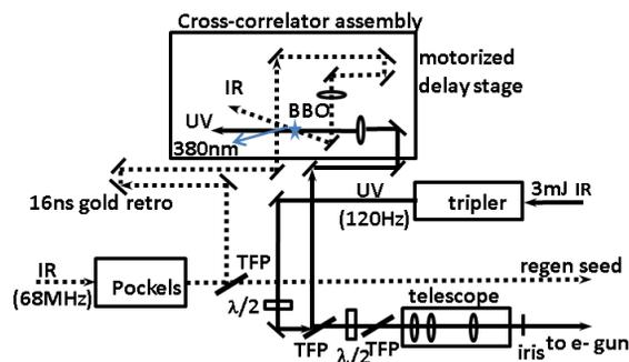
Figure 1: UV beam conditioning optics.
