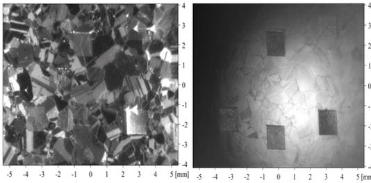
Figure 5: High-resolution photocathode images with 90° incident light (left) and 30° incident light showing laser processed areas and grain boundaries.
