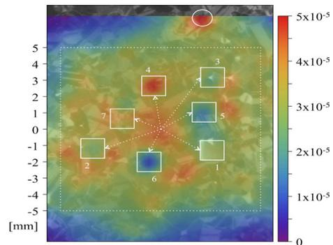
Figure 6: Quantum efficiency map across photocathode with 7 laser-processed spots indicated.
