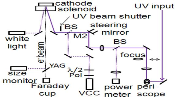
Figure 2: Schematic diagram of beam diagnostic system at the photocathode gun location.
