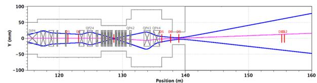
Figure 1: Plot of the vertical beam centroid (magenta) and the 10 sigma envelope (blue) along the transport line to the target. The raster magnets are located at about 128 m, the neutron shield wall at 139 m, and the target at 160 m.
