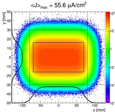
Figure 2: Predicted beam density at target surface.
