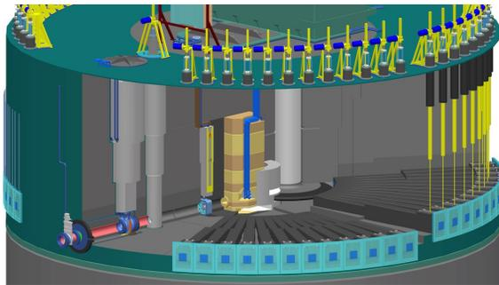
Figure 4: The target monolith. Beam arrives from the left, passing through the proton beam window, then the instrumentation plug, and finally hitting the edge of the rotating target located near the monolith center.
