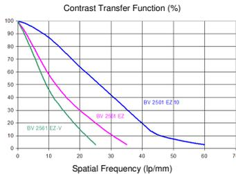
Figure 12: Spatial resolution of different image intensifier configurations: 2 MCPs green, 1 MCP pink and no MCP blue.
