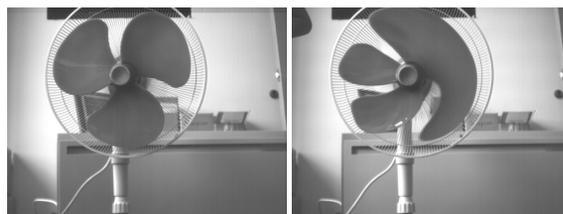
Figure 10: Images of a turning fan taken with a global shutter *left* and rolling shutter *right*.
