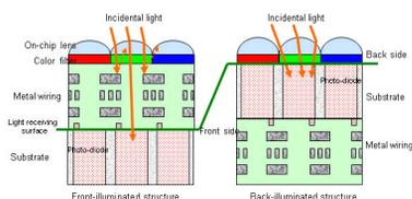
Figure 9: Structures of front and back illuminated CMOS sensors. Micro-lenses are also applied to concentrate the photons on the active area of the pixels.
