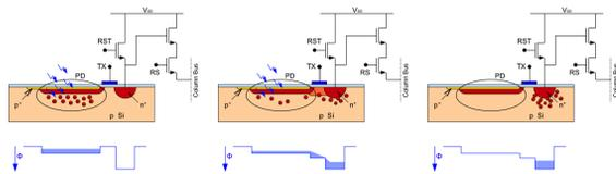
Figure 6: Signal integration and readout in a 4T CMOS.
