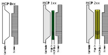
Figure 11: Layout of image intensifiers with 0, 1 and 2 MCPs.
