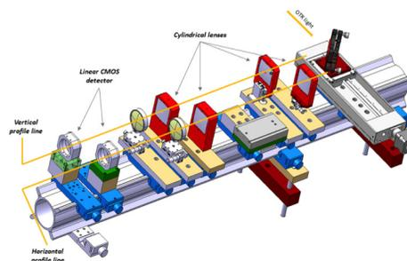
Figure 13: Rendering of the optical bench used for the LHC matching monitor.
