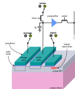
Figure 7: Sketch of a CID pixel.
