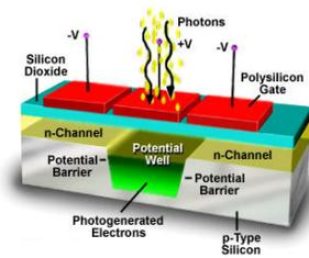
Figure 1: Structure of a CCD photo sensor based on a MOS capacitor.
