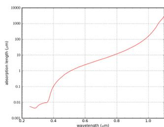
Figure 8: Light absorption in silicon vs. wavelength.
