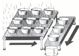
Figure 3: Integration and read-out principle of a CCD.
