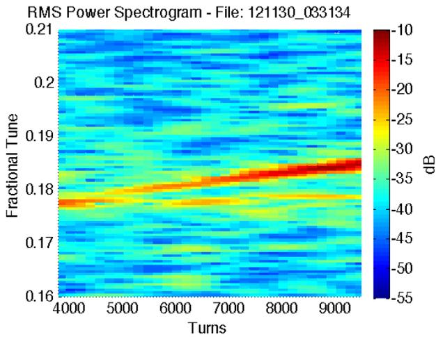
Figure 4: Measured RMS spectral power for a mode 1 excitation of the physical system. The barycentric mode 0 tune of 0.178 is weakly driven in this mode 1 excitation pattern. The chirp crosses the mode 1 tune (upper synchrotron sideband) of 0.183 near turn 8500. Noise floor below -55dB has been suppressed for clarity.
