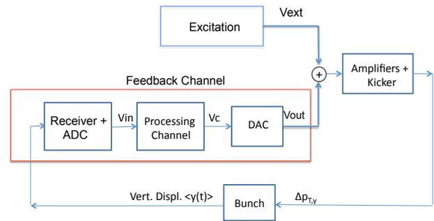
Figure 3: Loop topology for measuring beam dynamics changes due to feedback. An excitation signal  $V_{ext}$  drives the beam, while the closed loop feedback acts in response to the excitation. Time-domain samples of the excitation, and the beam response  $V_{in}$  are processed in both time and frequency domains.
