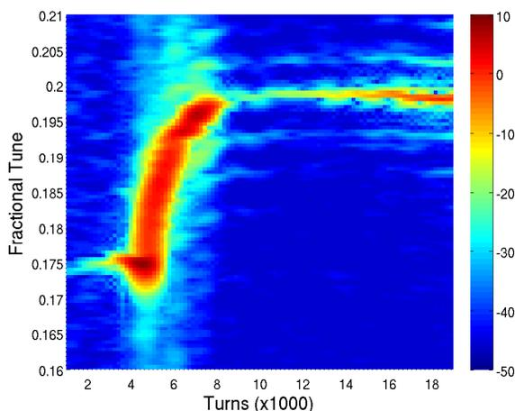
Figure 7: Frequency-domain spectrogram of unstable (no feedback) beam motion with charge loss. The machine chromaticity is ramped to zero at 2000 turns, resulting in mode 0 unstable beam. The dramatic tune shift is a sign of charge loss due to the unstable motion.
