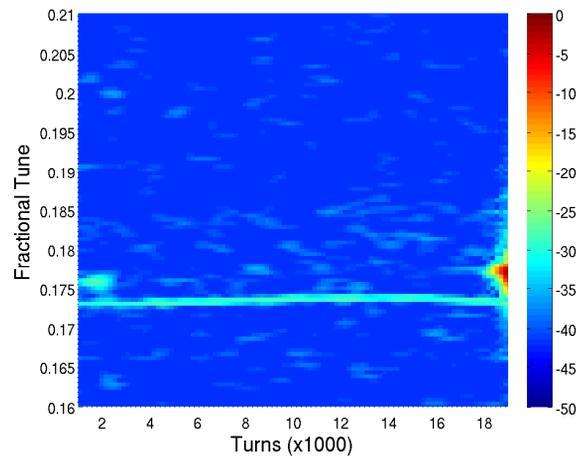
Figure 8: Identical injection case as Figure 7, but with feedback ON until turn 18,000. The stored beam is controlled vertically to 23  $\mu\text{m}$  RMS (1.5 ADC counts), unstable beam motion occurs after feedback gain is set to 0.
