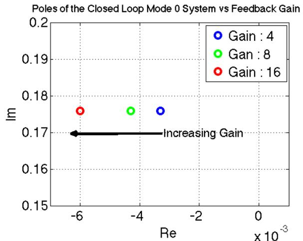
Figure 6: Pole locations of mode 0 under feedback control using three sets of physical measurements (three gains applied to the beam feedback). Using the three fitted simplified models, the increased damping of mode 0 created by increased gain is clearly quantified.
