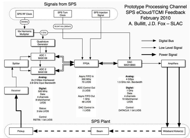
Figure 1: Block diagram of the demonstration system implemented at the SPS, showing the signal paths and the timing synchronization to the SPS. Not shown are the input phase equalization filters in the baseband path to correct for the pickup and cable transfer functions, and the back end equalizers used to correct the nonlinear phase response of the cable and kicker transfer functions [7].
