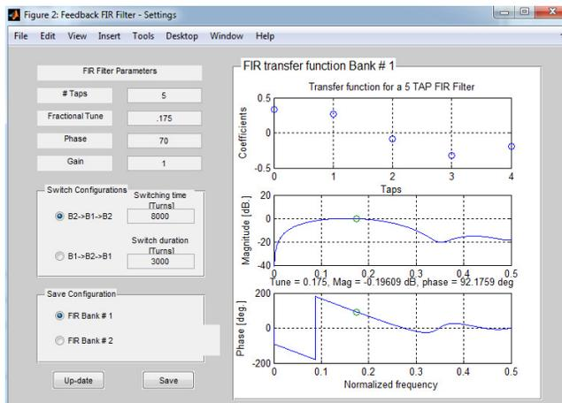
Figure 2: Typical control filter (bandpass filter at a nominal vertical tune of 0.175). The same filter coefficients are applied to each of the 16 control filters taken across the SPS bunch. With the use of the synchronizing signals it is possible to switch two independent filter sets “on the fly” to change feedback parameters during a machine cycle, allowing the system to track variations in tune, or to allow grow-damp or other time varying feedback studies
