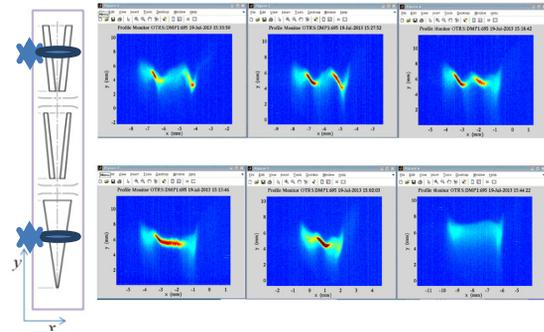
Figure 5: The action of a double slotted foil with varying separation (upper images), and a single foil of varying width (lower images), can be clearly seen with the XTCAV.
