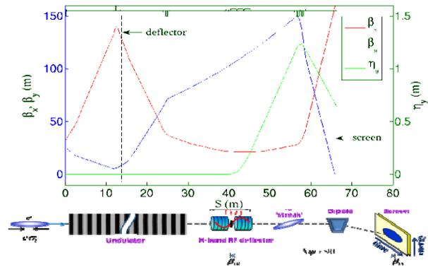
Figure 1: Optics between the XTCAV and the dump profile monitor screen.
