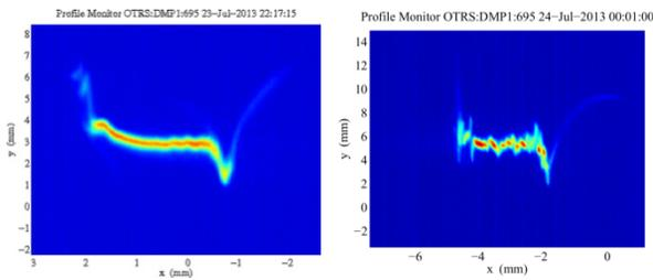
Figure 4: XTCAV images with laser heater on (left) and laser heater off (right), showing the microbunching instability growth.
