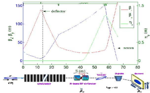
Figure 1: Optics between the XTCAV and the dump profile monitor screen.
