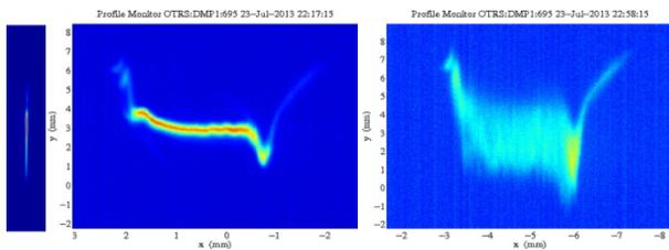
Figure 2: Profile monitor screen images for a 150 pC bunch at 4.7 GeV at the electron beam dump acting as a vertical energy spectrometer. At left the XTCAV is OFF; center image XTACV is ON and FEL is OFF; at right, XTCAV is ON and FEL is ON.
