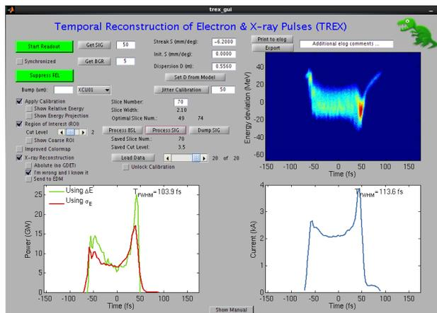
Figure 3: Screen shot of the user interface for analyzing the XTCAV image (top right) and calculating the peak current profile (bottom right) and the reconstructed x-ray temporal profile.
