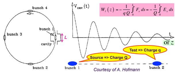
Figure 1: Illustration of the voltage induced by a bunch (bunch 1 in this example) going through a cavity. The bunch 2, at the distance  $z$  behind, will feel a longitudinal wake field given by the formula (more precisely, it is called wake function and it represents the response to a pulse of infinitely small length).
