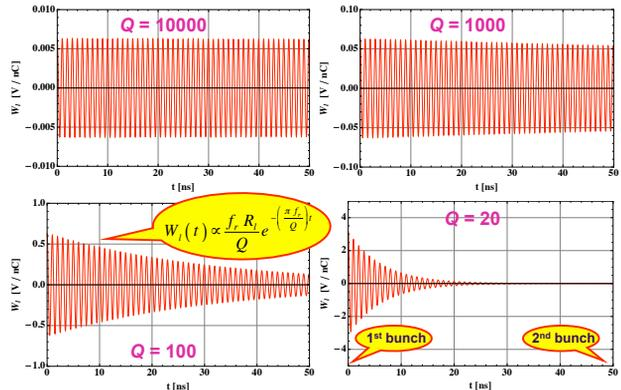
Figure 9: Impedance plots for a resonance with the resonance frequency  $f_r = 1$  GHz, shunt impedance  $R_l = 10 \Omega$ , for different values of quality factors  $Q$  and corresponding wake functions.
