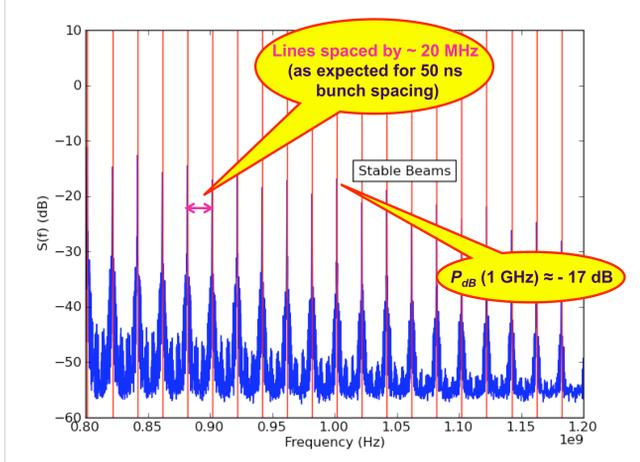
Figure 2: Power spectra measurements for LHC beam 1 on fill # 2261 (Courtesy of Themistoklis Mastoridis, Philippe Baudrenghien and Hugo Day).
