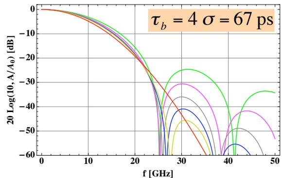
Figure 8: Power spectrum for a DLS bunch (5 mm rms, i.e. 67 ps at  $4\sigma$ ) assuming the bunch profiles of Fig. 5. To be compared to an LHC bunch (see Fig. 6).
