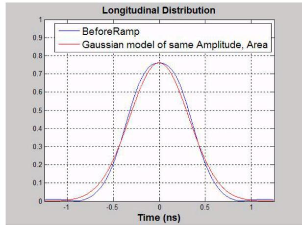
Figure 7: Longitudinal profile obtained by taking the inverse Fourier Transform of the measured spectrum before the ramp (see Fig. 2a; Courtesy of Themistoklis Mastrodis and Philippe Baudrenghien).
