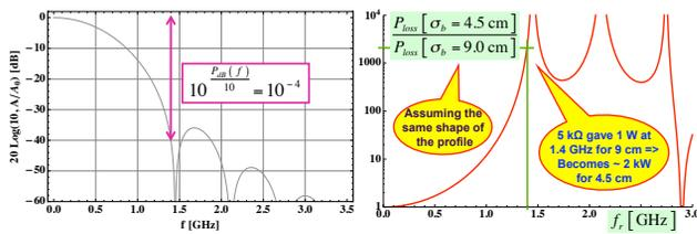
Figure 10: Theoretical (see Fig. 6 with  $n = 3$ ) longitudinal bunch spectrum for the case of a LHC bunch in 2011 (9 cm rms bunch length) and power loss increase for the case of a bunch two times shorter (4.5 cm rms) assuming the same shape.
