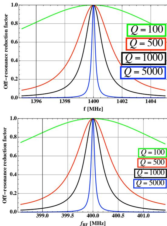
Figure 11: Off-resonance effect on the power loss, applied to the case of Fig. 10, vs. (a) the resonance frequency and (b) the RF frequency (assuming the resonance frequency at 1.4 GHz).
