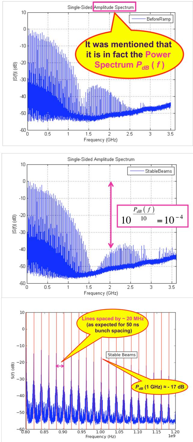
Figure 2: Power spectra measurements for LHC beam 1 on fill # 2261 (Courtesy of Themistoklis Mastoridis, Philippe Baudrenghien and Hugo Day).
