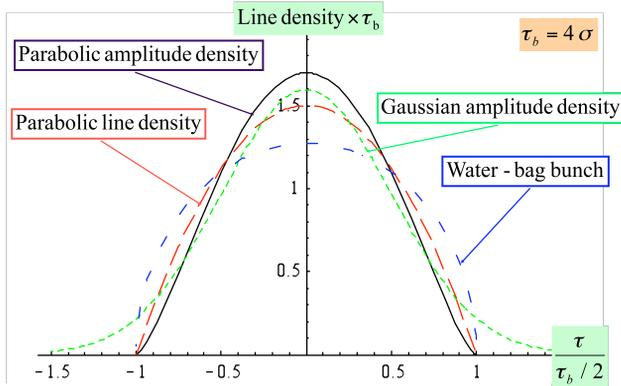
Figure 3: Longitudinal profiles of four typical (theoretical) distributions.
