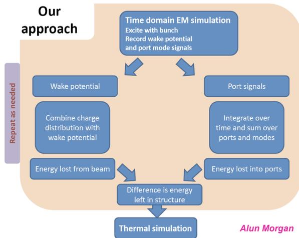
Figure 13: Approach being currently applied at the DLS to study the beam-induced RF heating [9].
