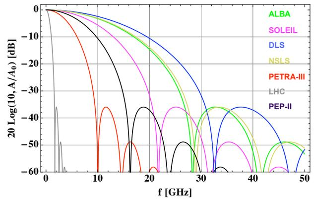
Figure 12: Comparison between the different longitudinal beam power spectra, revealing the frequency ranges of interest for the different machines.
