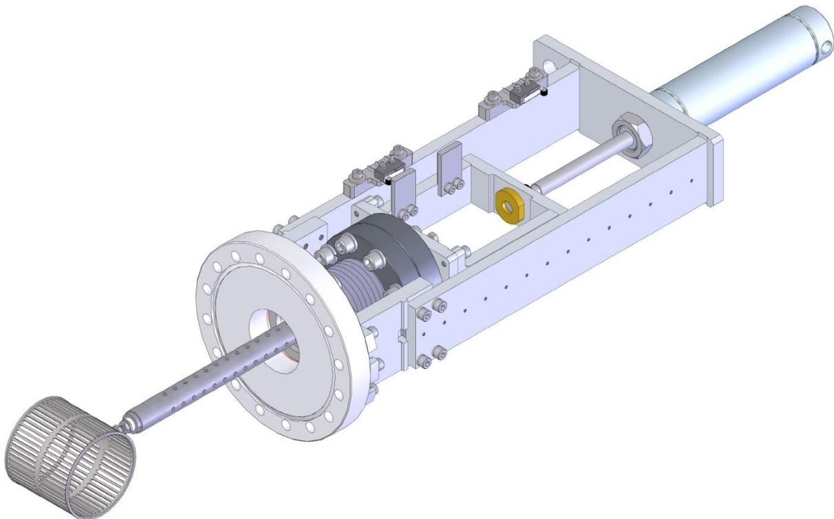
Figure 2: A SolidWorks model of a VECC RF shield.
