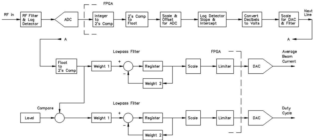
Figure 4: The data flow through the log detector, ADC, DACs and 50 MHz signal processing pipeline.
