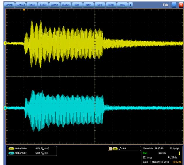
Figure 3: Signals from the two the RF Shields closest to the VECC e-gun. The beam current is 2.8 mA peak and the pulse width is 520 ns.
