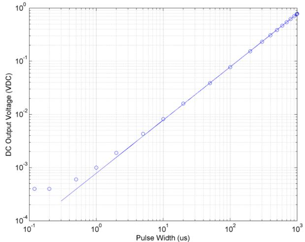
Figure 6: The response of the electronics to a pulsed signal.
