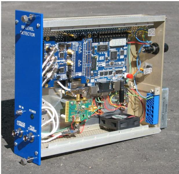
Figure 7: The prototype module is built into a double width NIM module.
