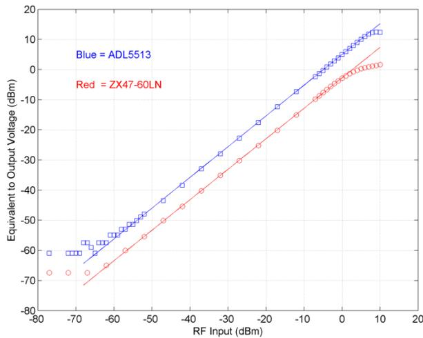
Figure 5: The response of the electronics for two different log detectors. The response of the ZX47-60LN has been decreased by 10 dB for clarity.
