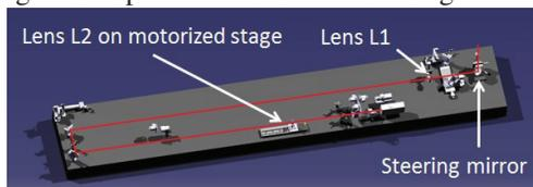
Figure 4: Optical line based on focusing lenses.
