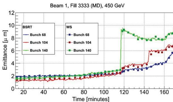
Figure 7: Comparison between BSRT and Wire Scanner.
