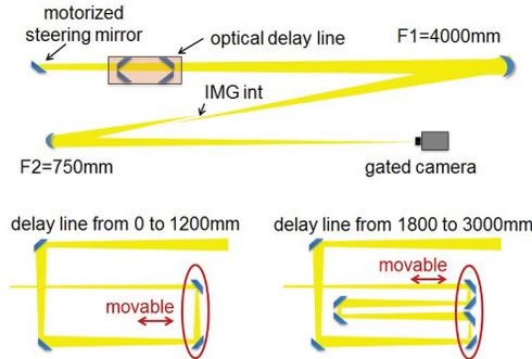
Figure 2: Sketch of the optical line with spherical mirrors.
