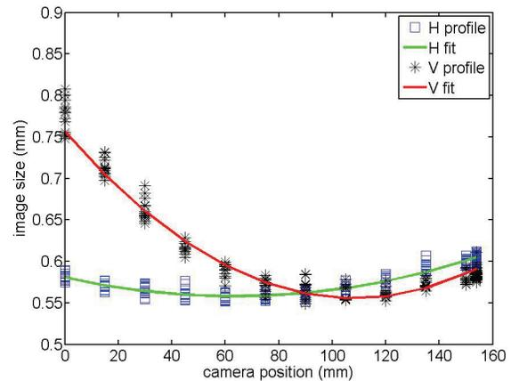
Figure 6: Example of lab measurements: image size of a circular iris for different camera positions. The points are fitted with a parabola, whose minimum corresponds to the image plane.
