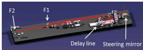
Figure 3: Optical line based on focusing mirrors.
