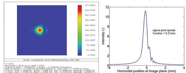
Figure 5: Image and horizontal profile as scored by Zemax (POP mode) at the image plane, for a single proton traveling through the D3 dipole.
