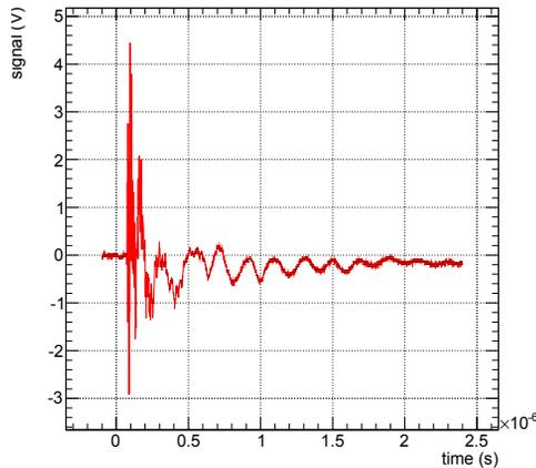
Figure 8: Uncalibrated electromagnetic field as detected by the oscilloscope after passing through 10 m long cable and 13 db attenuator. This whole chain was later calibrated to obtain absolute values of the electromagnetic fields reaching in average 7 kV/m.
