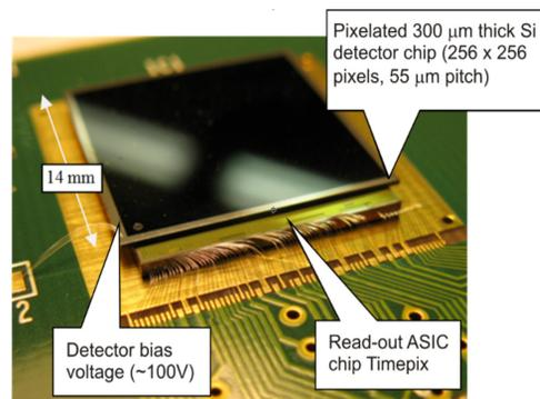
Figure 1: Timepix read-out ASIC chip with  $300 \mu\text{m}$  thick silicon sensor.
