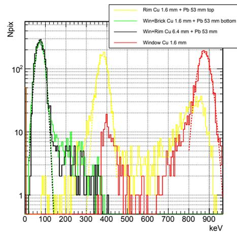
Figure 6: Energy spectra collected from areas of Timepix detector protected by various shielding materials (see the legend for details). This corresponds to detector signal presented in Fig. 5. During the shot, each pixel detected a pile-up of energy deposits from many particles. The shielded detector however survived strong radiation and electromagnetic fields (of 7 kV/m), which was the primary goal of the study.
