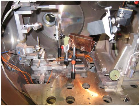
Figure 4: Experimental setup at PALS facility inside the target vacuum chamber. The PALS 700 J laser pulse is focused by the large lens on the right-hand side onto the solid target in the mount on the left hand side. In front of the Timepix copper shielded box, there is a 54 mm thick lead brick, covering half of the detector active area, as viewed from the target.
