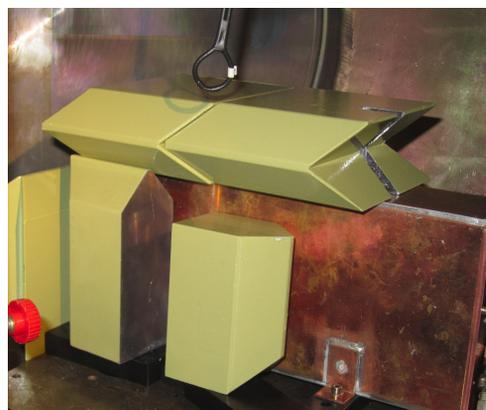
Figure 7: The black wire loop at the top of the figure shows the antenna used for measurements of the electric fields inside the vacuum chamber. The shielding of the coaxial cable of the antenna is connected to the vacuum chamber walls.
