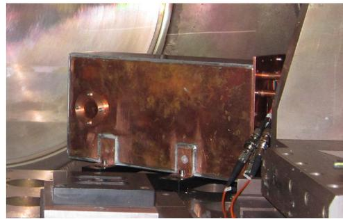
Figure 3: The copper shielding of the whole detector setup. The Timepix detector is positioned behind the round copper ring, which enables to mount different shielding windows. Only the optical cables penetrate through the shielding on the right-hand side.
