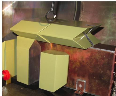
Figure 7: The black wire loop at the top of the figure shows the antenna used for measurements of the electric fields inside the vacuum chamber. The shielding of the coaxial cable of the antenna is connected to the vacuum chamber walls.
