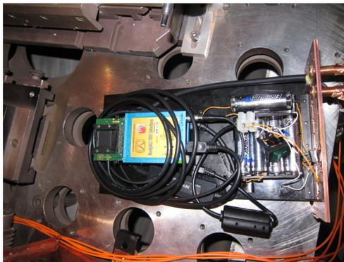
Figure 2: The optics-only setup with removed copper shielding. The Timepix detector (black square) is connected to the USB readout unit FitPix (blue), which is read out by commercial off-the-shelf USB optical cable. The optical converter (little black box) and FitPix are powered by standard Lithium batteries.
