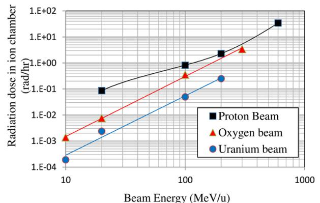
Figure 2: Instant gamma ray dose (rad/hr). Loss is normalized to 150W/150m. Proton is listed as reference.
