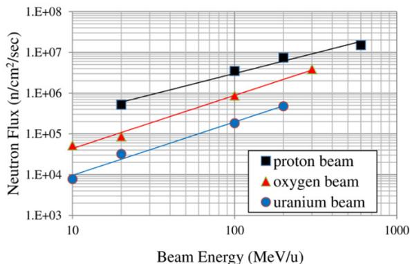
Figure 3: Neutron Flux (n/cm<sup>2</sup>/sec). Loss is normalized to 150W/150m.
