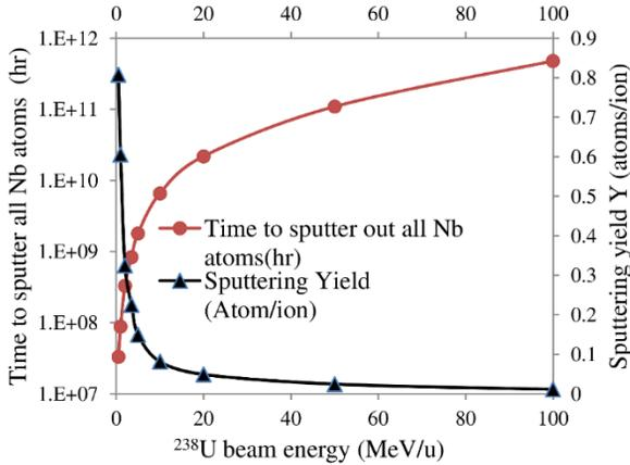
Figure 4: Estimation of damage time to HMR by slow loss induced sputtering. Damage time (red circles) is calculated by Equation (2) in unit of hours.
