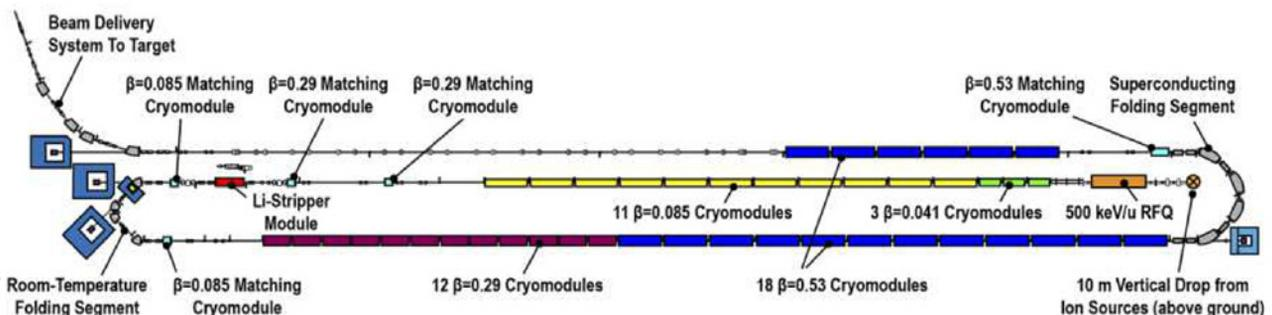
Figure 1: Schematic layout of FRIB driver linac. The specific energy for 238U is 0.5-17 MeV/u at LS1, 17 - 150 MeV/u at LS2, and 150 MeV -200 MeV/u at LS3.
