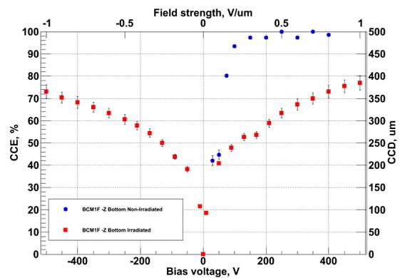
Figure 6: Charge collection efficiency for BCM1F diamond before and after irradiation.
