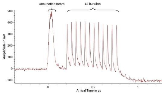
Figure 2: Beam losses after injection. The detected beam losses originate from unbunched beam and 12 injected bunches separated by 50 ns.
