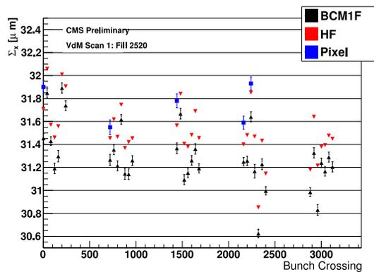
Figure 5: Measured beam width as a function of bunch crossing for BCM1F and HF. The beam width was obtained by Van der Meer scans.
