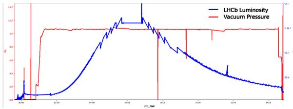
Figure 4b: Luminosity and vacuum pressure measurements for LHCb.
