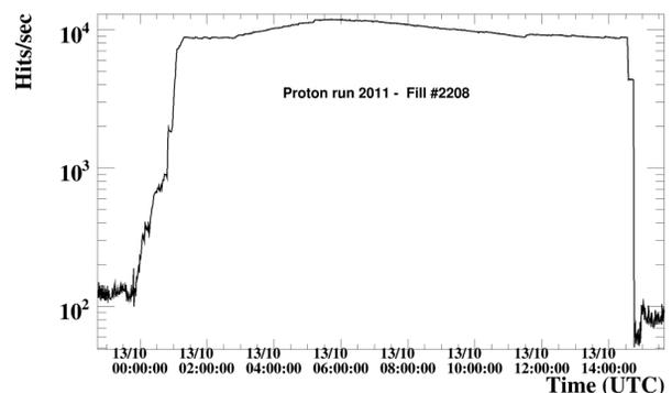
Figure 4a: Scaler rates over one LHC fill measured with scCVD sensor near to LHCb.
