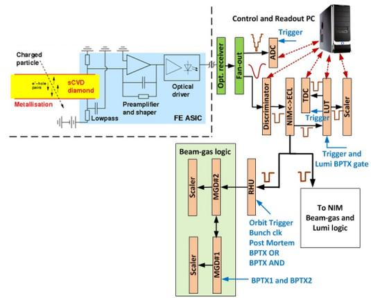
Figure 3: BCM1F readout system consisting of diamond sensors, ASICs, optical drivers and back-end modules.
