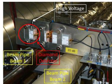
Figure 1: Diamond detector installed above the beam pipe.
