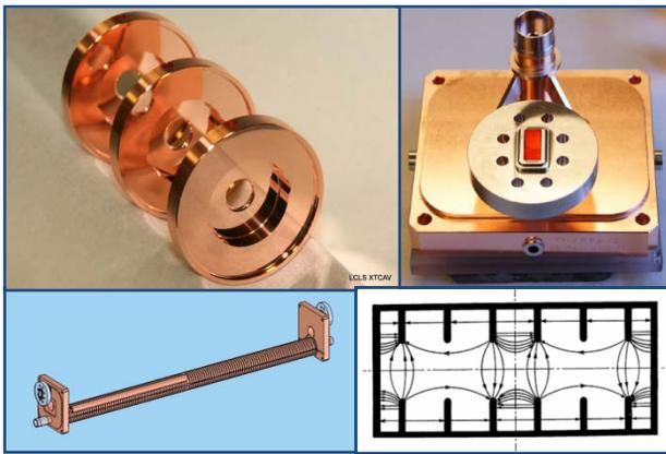
Figure 2: Fabrication details of the  $\text{HEM}_{11} 2\pi/3$  X-band transverse deflecting structure, showing the individual cups before bonding, and the coupler.
