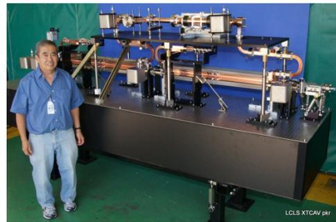
Figure 4: The deflecting structures preassembled and aligned on an optical bench before installation.
