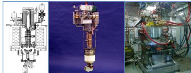
Figure 5: SLAC XL4 X-band klystron and assembly.
