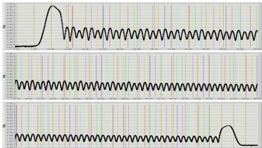
Figure 3: Measured electric field amplitude inside the deflector after tuning.
