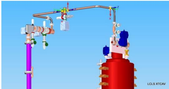
Figure 6: X-band waveguide layout from the klystron to the tunnel penetration.
