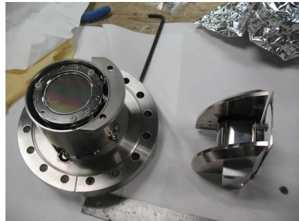
Figure 4: The electron collector with an MCP amplifier (left) and the in-vacuum magnet (right).
