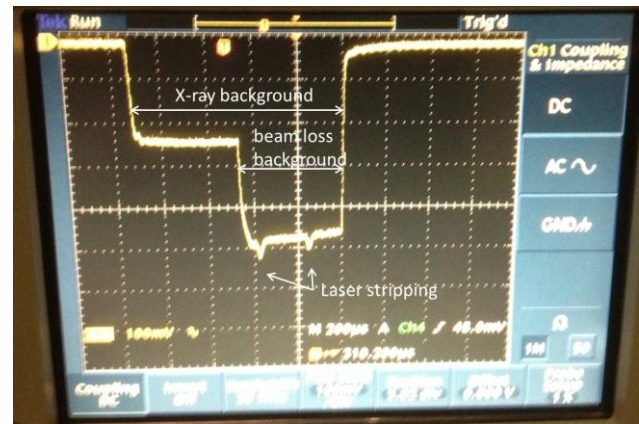
Figure 5: A typical raw signal from the electron detector.
