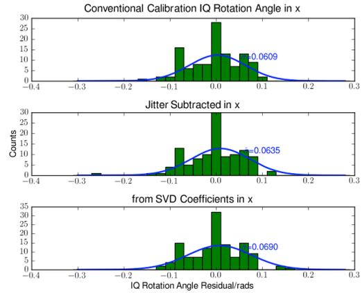
Figure 3: Horizontal CBPM calibration IQ rotations  $\theta_{IQ}$ .
