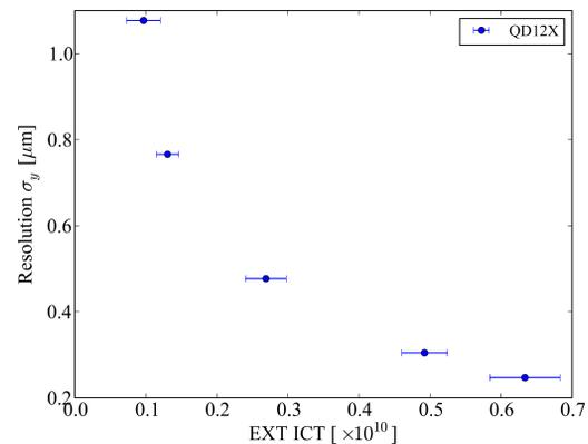
Figure 1: Resolution measured at different bunch charge settings measured by the extraction line current transformer.
