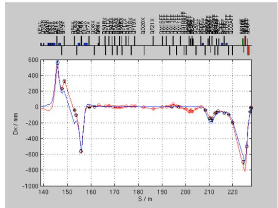
Figure 8: Example of horizontal dispersion measurement.
