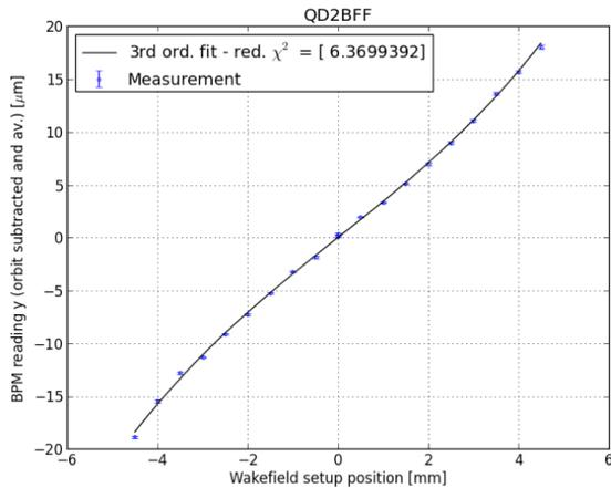
Figure 5: Example of a wakefield kick measurement.
