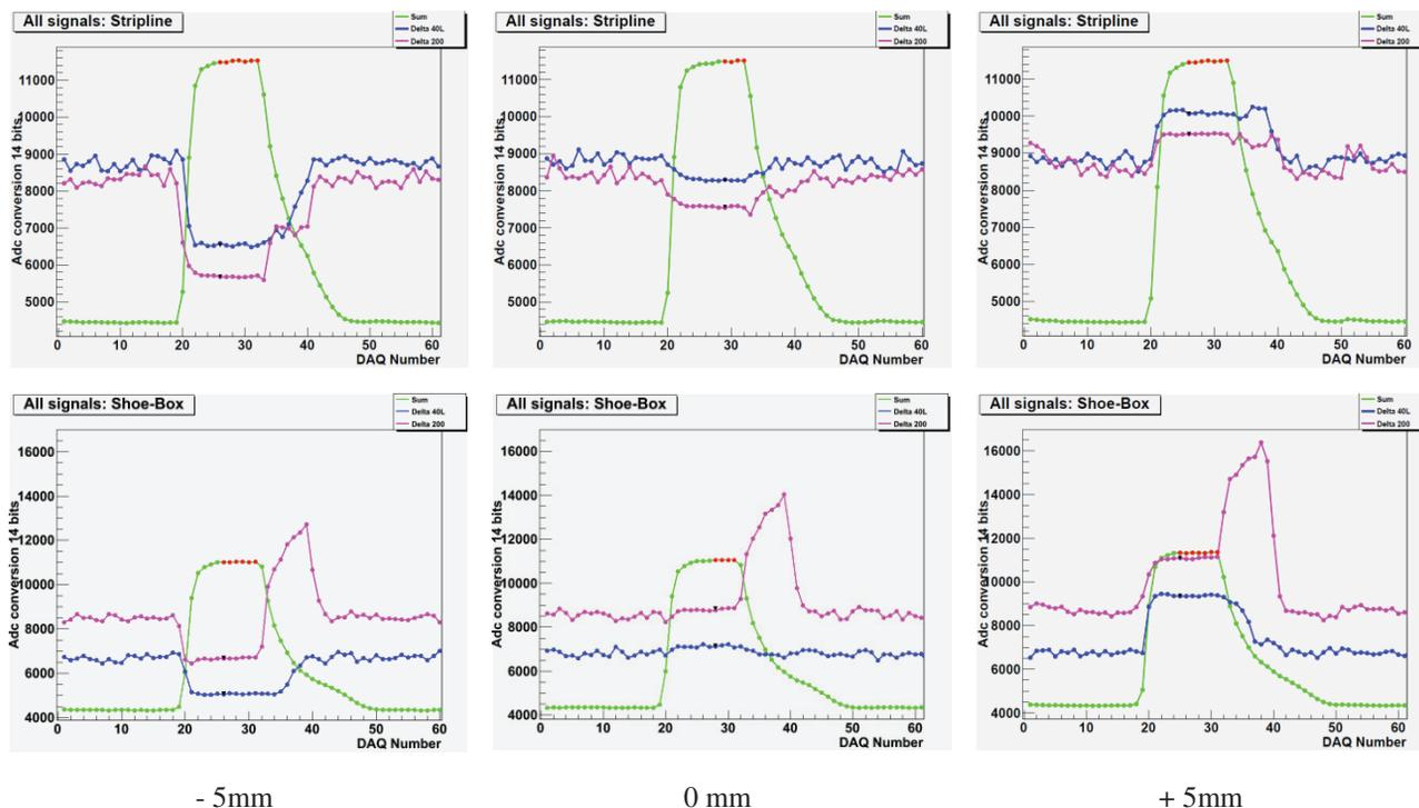
Figure 7: Data acquisitions, without (0mm) and with  $\pm 5$ mm beam-bumps.
