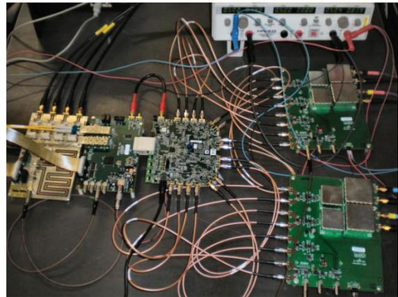
Figure 3: Hardware of the Front-End prototype, which includes 2 Log-Amp boards, 1 octal-ADC, 1 calibrator and 1 FPGA-based acquisition board.
