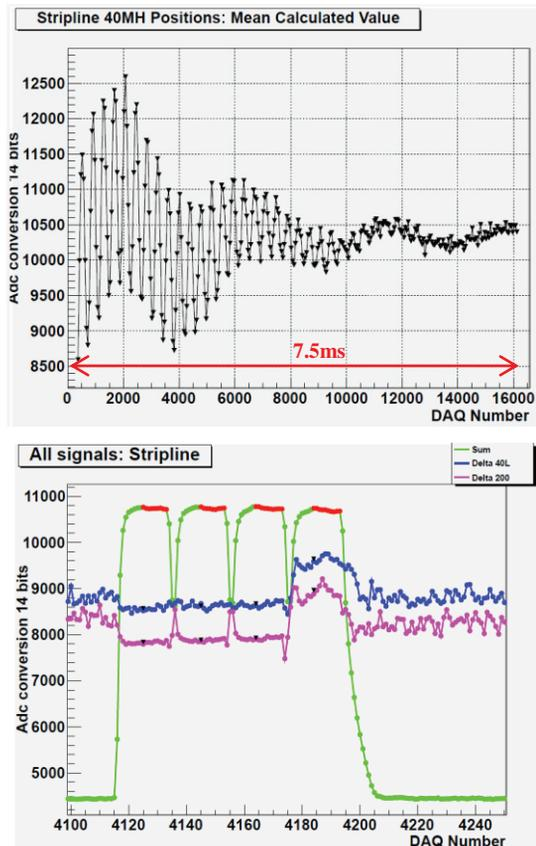
Figure 5: Proton beams. (Top) Single-bunch horizontal injection oscillations. (Bottom) Intensity and position signals of 36 bunch-batches with 50 ns-spacing, during the 4<sup>th</sup> batch injection.
