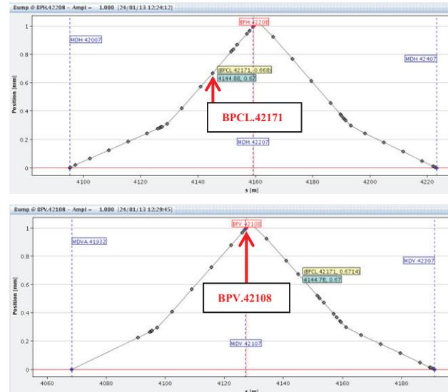
Figure 6: Local beam bumps, either in the horizontal or the vertical plane, are generated using beam corrector elements.
