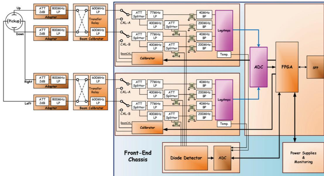
Figure 2: MOPOS Front-End electronics diagram.
