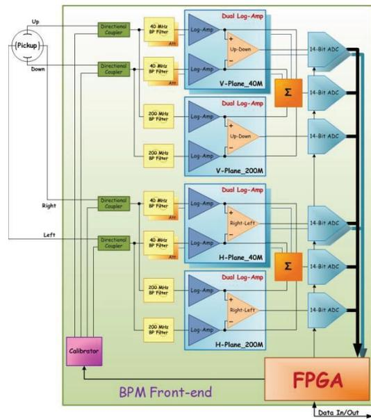
Figure 1: Front-End Prototype block diagram.
