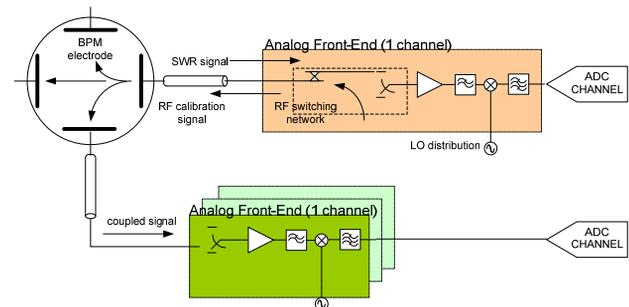
Figure 3: Measurement of BPM button coupling and SWR.
