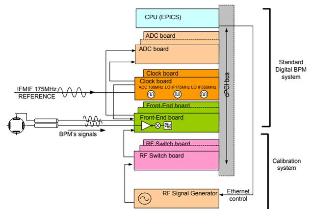
Figure 1: General layout of the BPM electronics.
