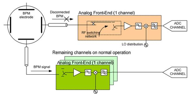
Figure 2: Calibration of the RF electronics.
