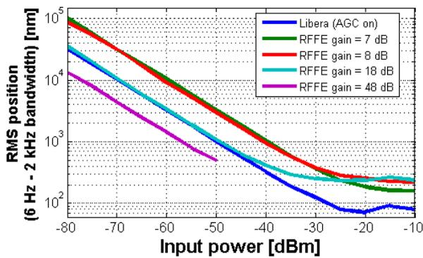
Figure 3: RMS resolution (6 Hz to 2 kHz bandwidth) vs. input power.
