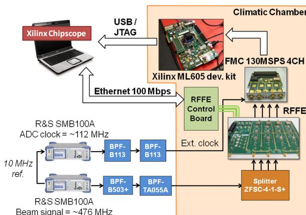
Figure 2: Experimental setup for the Sirius BPM electronics prototype evaluation.
