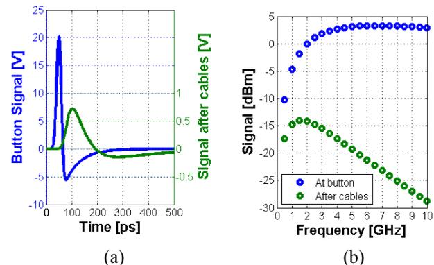
Figure 1: Simulation of the RF voltage signal at button pick-ups and after LMR195 cables of a 500 mA multi-bunch beam with ideal 100% filling: (a) Time-domain; (b) Frequency-domain (RF frequency harmonics).
