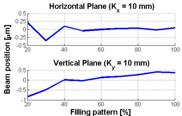
Figure 5: Filling pattern dependence for a 100 mA centered beam.
