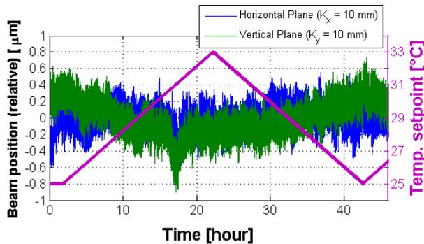
Figure 6: Temperature dependence for a 500 mA centered beam (10 Hz data rate).
