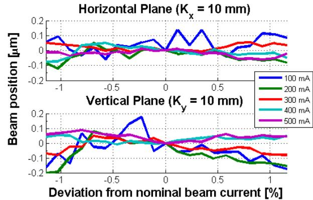
Figure 4: Short-range beam current dependence for centered beam in different beam current scenarios.
