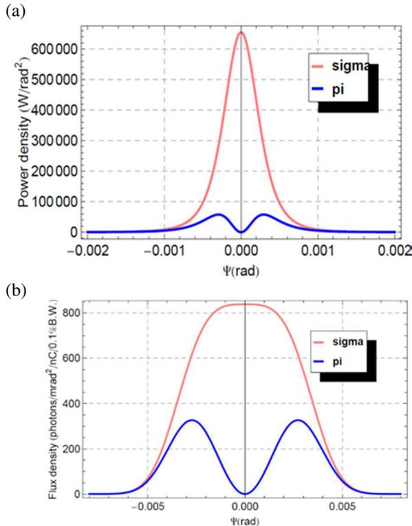
Figure 7:  $\sigma$  component and  $\pi$  component of (a) the emission power density and (b) spectral angular density of flux [ $\text{photons/s/rad}^2/0.1\% \text{band width/A}$ ] from the bending magnet.
