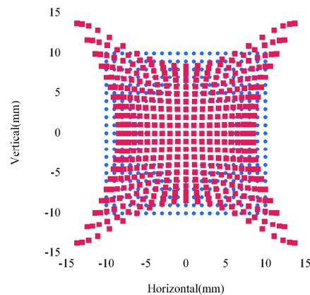
Figure 3: Mapping of beam position using the log-ratio method.
