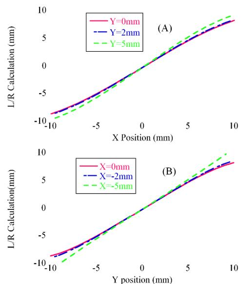
Figure 4: The beam position v.s. the result of the LR calculation method when we fixed a vertical position and changed the horizontal position (A) and when we fixed a horizontal position and changed the vertical position (B).
