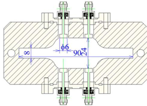
Figure 2: BPM monitor chamber.
