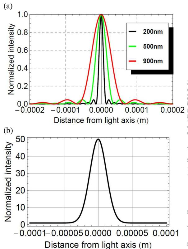
Figure 6: (a) A pattern of the Fraunhofer diffraction at the extraction mirror of the SR with λ = 200nm, 500nm and 900nm. (b) The convolution of the quantum efficiency of the camera and the Fraunhofer diffraction pattern of λ = 200nm - 900nm.
