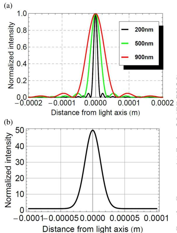
Figure 6: (a) A pattern of the Fraunhofer diffraction at the extraction mirror of the SR with λ = 200nm, 500nm and 900nm. (b) The convolution of the quantum efficiency of the camera and the Fraunhofer diffraction pattern of λ = 200nm - 900nm.
