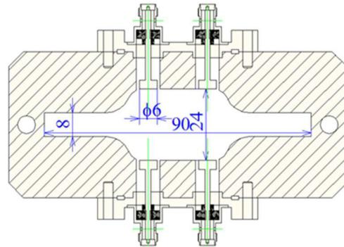
Figure 2: BPM monitor chamber.
