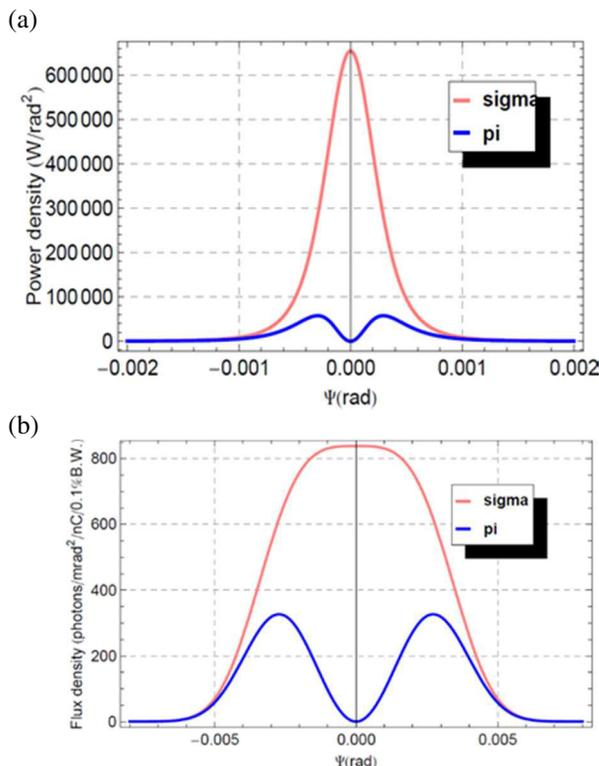
Figure 7:  $\sigma$  component and  $\pi$  component of (a) the emission power density and (b) spectral angular density of flux [photons/s/rad<sup>2</sup>/0.1%band width/A] from the bending magnet.
