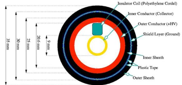
Figure 8: Ion chamber for the beam loss monitor.
