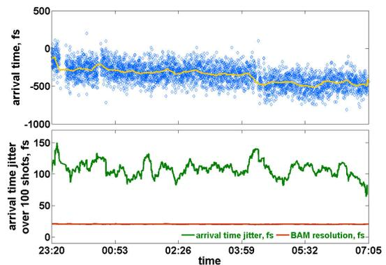
Figure 6: (upper plot) BAM drift measurement with the button pickup at mean charge 130 pC and with mean resolution 20 fs.
