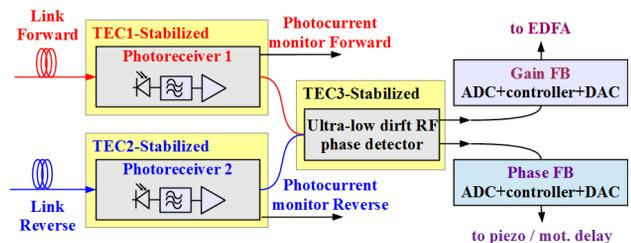
Figure 2: Block diagram of the low drift RF phase detector, used for stabilization of the pulsed BAM link.
