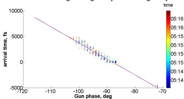
Figure 7: Bunch arrival-time as a function of the gun phase with slope 310 fs/deg.
