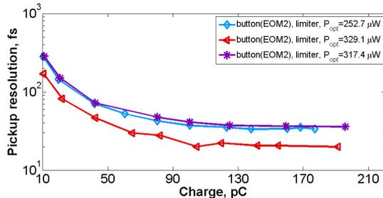
Figure 4: Pickup resolution dependence on the charge.
