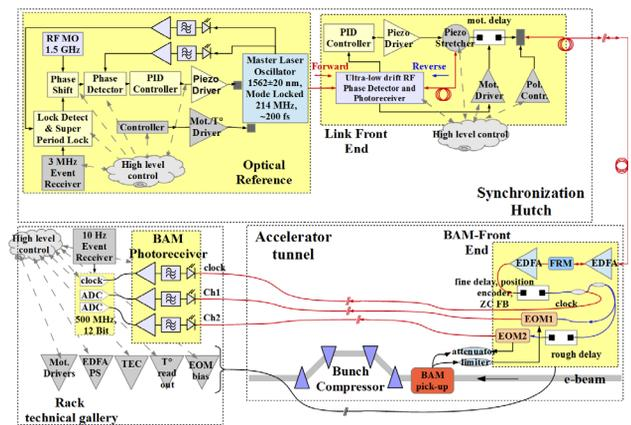
Figure 1: Layout of BAM and its stabilized pulsed optical reference.
