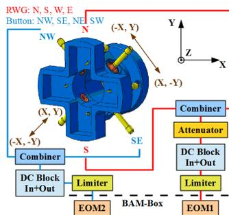
Figure 3: Layout of the pickup and RF-Front-End. Map for the orbit scans.
