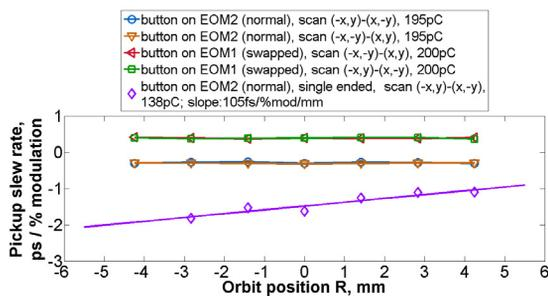
Figure 5: Orbit dependence of the button pickup slew rate.
