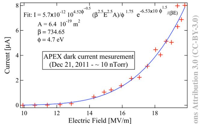
Figure 4: Dark current measurements as function of electric field in the gun.
