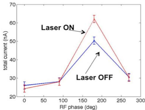
Figure 5: Measurements of 10 nA electron beam current using a lock-in amplifier.
