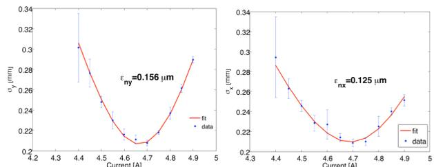
Figure 8: First thermal emittance measurement of  $\text{Cs}_2\text{Te}$  cathode.
