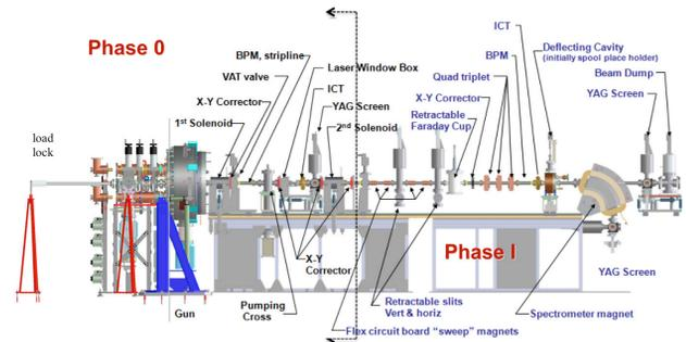
Figure 1: APEX layout for phase 0 and I.
