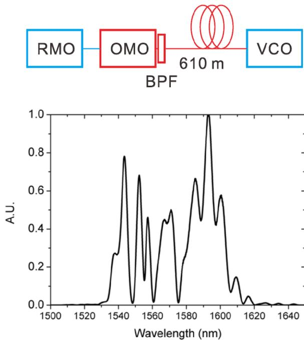
Figure 2: Experimental scheme and the spectrum of optical master oscillator.
