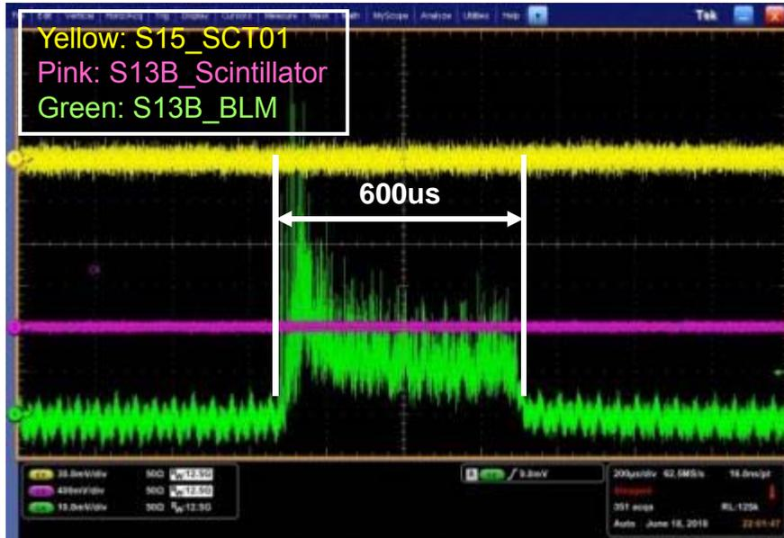
The plastic scintillation monitor with less X-ray sensitivity is employed to measure the beam loss.
