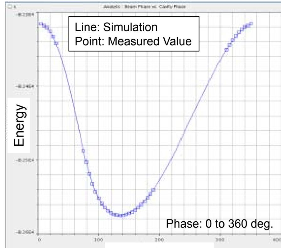
In order to seek an adequate set-point, matching is implemented by the phase scan. The set-point is determined from the best matching point between the measurement and model simulation.
