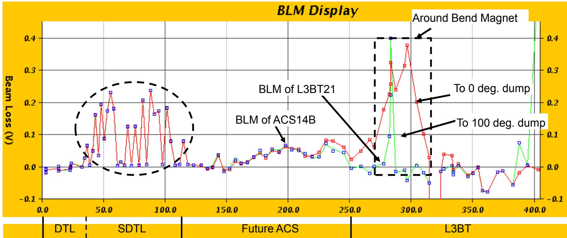
X-ray emitted from the SDTL cavities is detected by the BLM.
