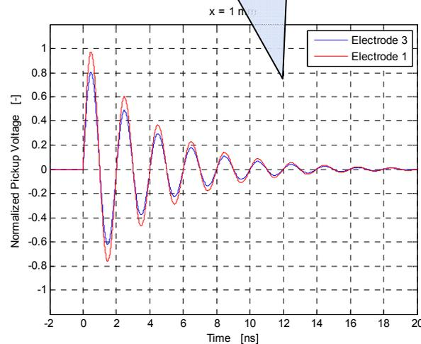
Ringing filter output: Pulse stretching improves resolution (reduces digitizer jitter impact).
