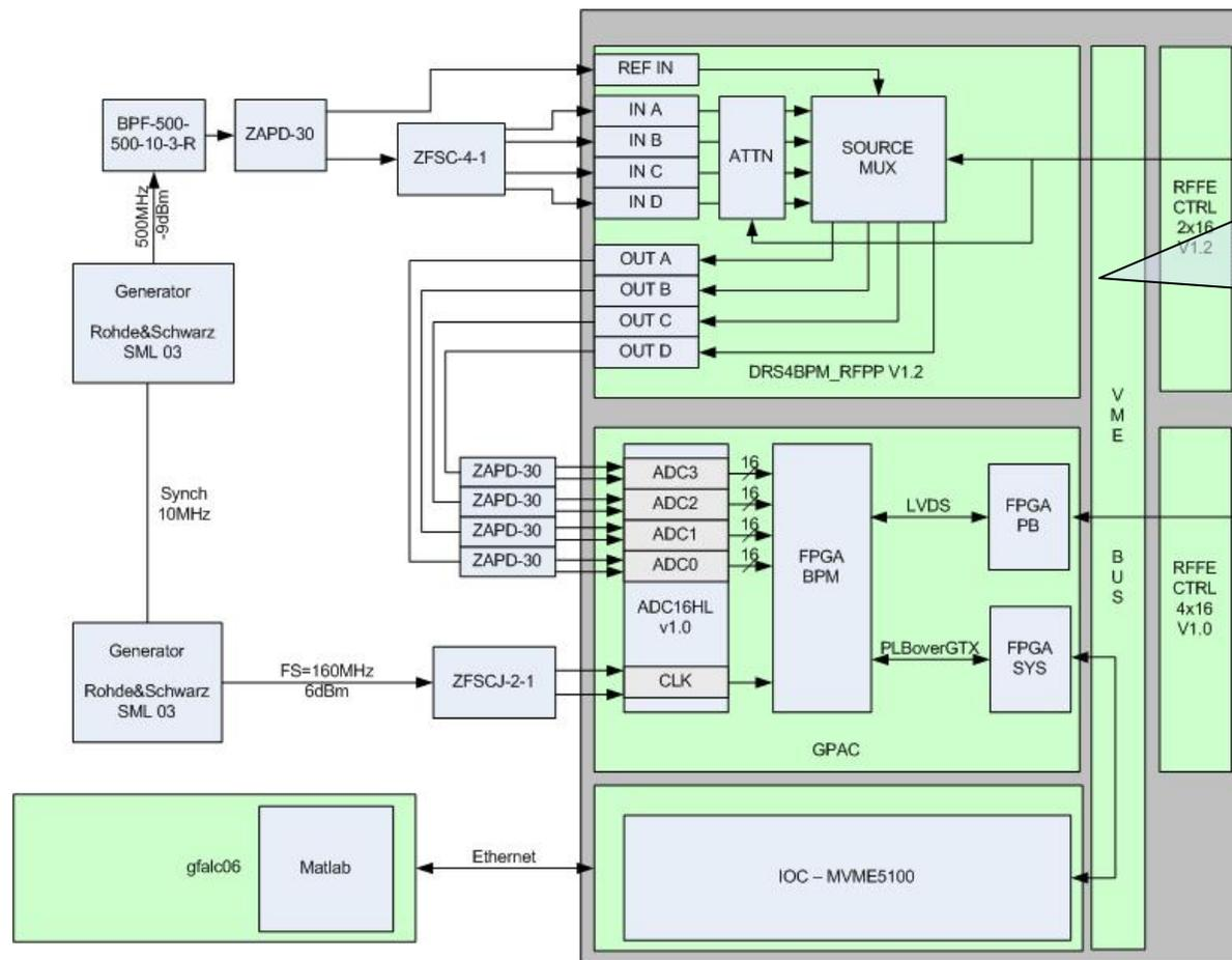
PSI modular BPM electronics: Using SwissFEL test injector 500MHz resonant stripline RFFE & E-XFEL cavity BPM ADC for tests (DDC, ...), until dedicated new SLS ADC & RFFE are ready.
