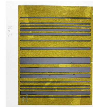
Diamond+Au mask Minimum slit width 10μm
