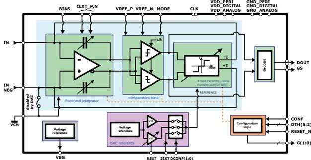
Figure 3: Diagram of a single A/D channel.
