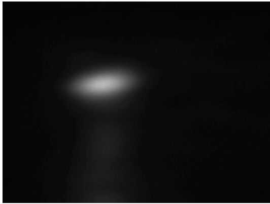
Figure 4: Electron beam profile measured using SR monitor. The stored beam current is 7 mA single bunch. Deduced horizontal beam size is less than 1 mm.
