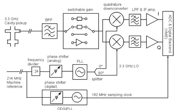
Figure 1: Simplified downconverter block diagram (one channel).
