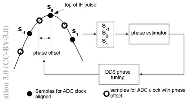
Figure 7: Principle of sampling phase alignment feedback loop.
