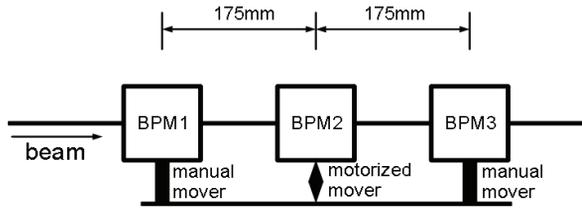
Figure 10: BPM (Ø10mm) pickup arrangement.
