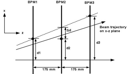
Figure 12: BPM resolution measurement using 3 cavities.
