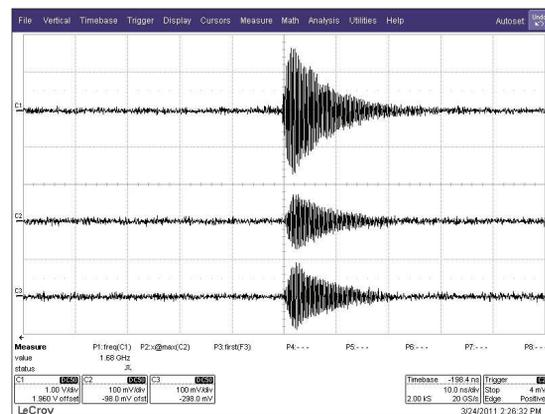
Figure 5: Cavity signals at input of RFFE (timescale: 10ns/div).
