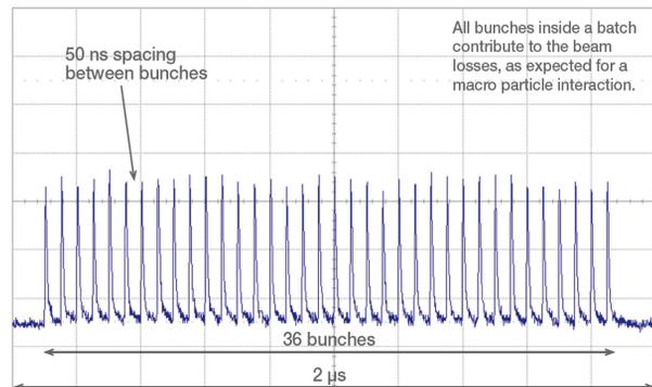
Figure 6: 2  $\mu$ s zoom; the bunches are separated by 50 ns, 36 bunches form a batch. It is remarkable that all bunches inside a batch contribute to the beam losses, as expected for a macro-particle interaction.
