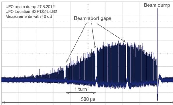
Figure 3: 500  $\mu$ s zoom; UFO location in Point 4, recorded in the collimation area in Point 7 with a 10x10x0.5 mm<sup>3</sup> diamond detector with 40 dB signal amplification. The length of the loss is about 0.5 ms. Beam abort gaps are clearly resolved.
