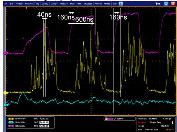
Figure 7: Signals from a gas proportional monitor (blue) and plastic scintillation monitor (yellow) at SDTL13 section, during beam operation with chopped beam. Time scale is zoomed up to 400nsec/div. The beam current signal with a current transformer is also shown (magenta).
