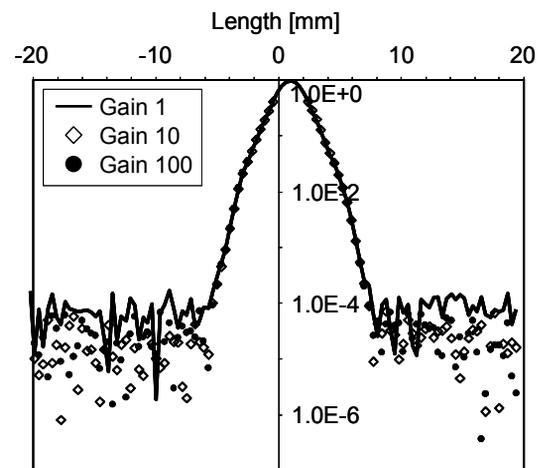
Figure 3: Vertical beam profile at ACS03. RMS spot size is almost 1.0 - 2.0 mm and dynamic range reaches  $10^4$ .
