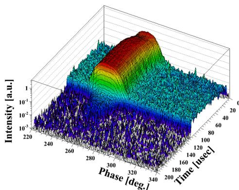
Figure 9: First beam data of J-PARC 181 MeV longitudinal distribution taken at the beam commissioning in Oct. 2012.
