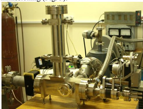
Figure 8: Bunch shape monitor for J-PARC Linac. The monitor was tested in INR test stand.
