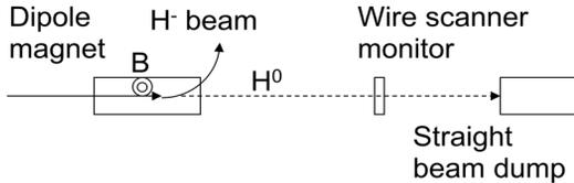
Figure 5: Method of H<sup>0</sup> particle measurement. H<sup>0</sup> was observed with carbon plate in wire scanner at the straight beam dump with a bending magnet on.
