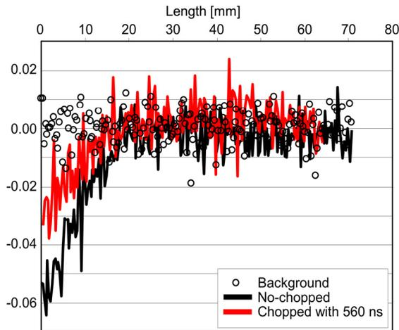
Figure 6: Signal from H<sup>0</sup> taken by carbon plate in wire scanner.
