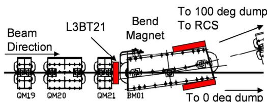
Figure 2: Gas proportional BLMs are installed to measure the beam loss caused by protons. Red bars are location of BLMs.
