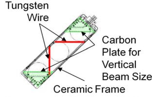
Figure 4: Head of Wire Scanner. Beam size can be measure by the wide carbon plate.
