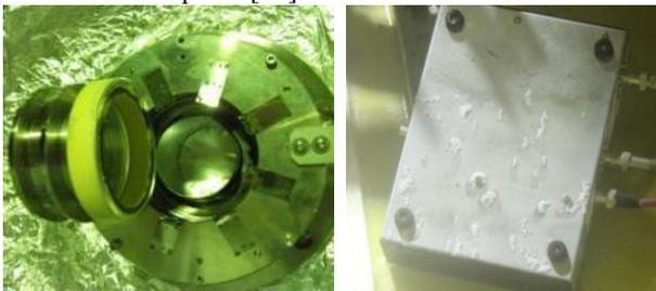
Figure 11: Detachment of the brazing section between the ceramic tube and stainless duct of S/FCT monitor (left). And corroded pre-amplifier boxes on the floor by strong alkaline (right).
