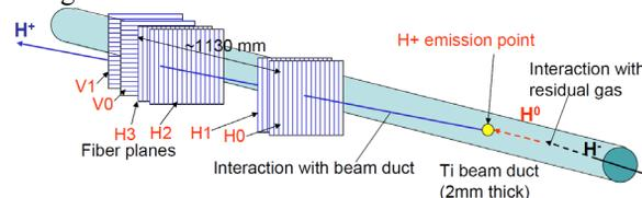
Figure 10: Beam loss tracking system by fast trigger scheme.
