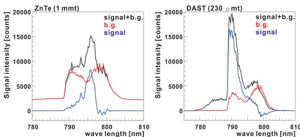
Figure 7: Signal intensity spectra of BCD measurement via 1 mm thick ZnTe (left) and 230  $\mu\text{m}$  thick DAST (right) Pockels EO crystals. Average bunch charge is fixed as 0.28 nC.
