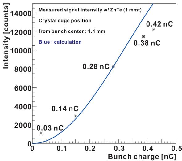
Figure 6: Dependency of the EO signal intensities on the bunch charge.
