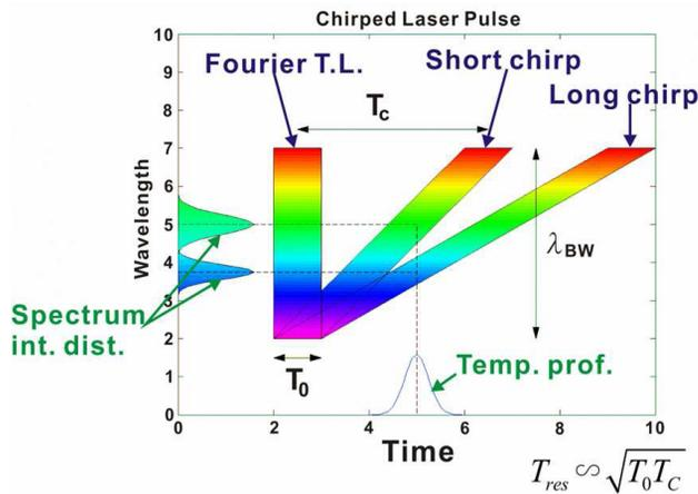
Figure 2: EO-encoded spectra with different chirp rate.
