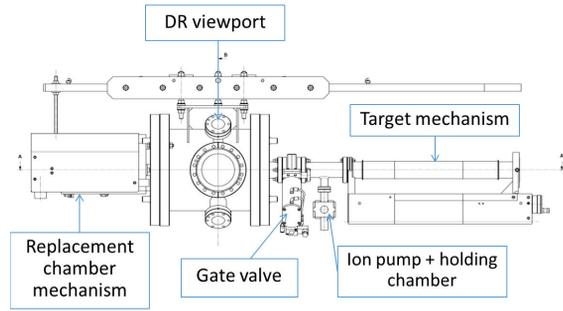
Figure 5: Overview of the DR tank. Electron beam direction is into the page [23].
