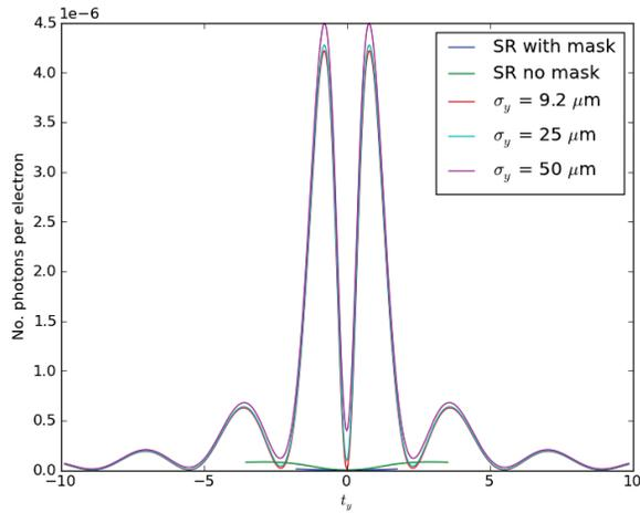
Figure 3: Comparison of DR vertical projections and SR background at  $E = 2.1$  GeV,  $\lambda = 400$  nm and  $a = 0.5$  mm.
