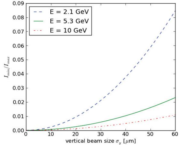
Figure 2: Sensitivity to beam size at different beam energies for  $\lambda = 400$  nm,  $a = 1$  mm and  $\sigma_y = 50$   $\mu\text{m}$ .
