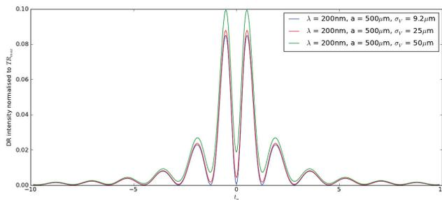
Figure 1: DR angular distributions at different beam sizes for  $E = 2.1$  GeV,  $a = 0.5$  mm and  $\lambda = 200$  nm.
