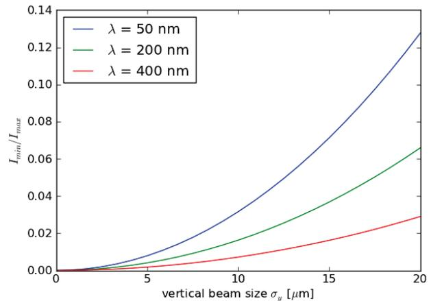
Figure 8: Sensitivity to beam size at  $\lambda = 50$  nm (phase 2) and  $\lambda = 200$  nm, 400 nm (phase 1). The target aperture is 0.2 mm.
