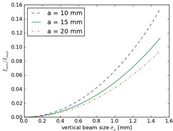
Figure 9: Sensitivity to beam size for the LHC at different target apertures.
