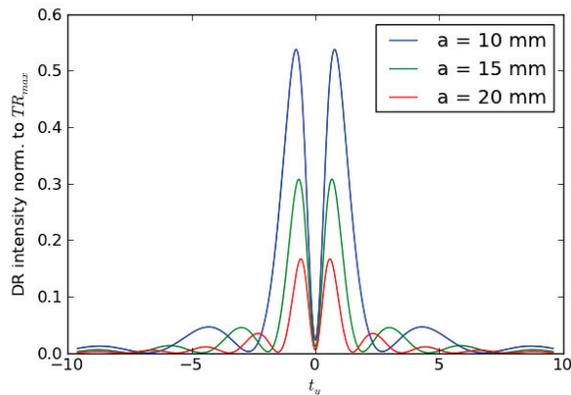
Figure 10: DR angular distributions at different target aperture sizes for the LHC ( $\lambda = 10.3 \mu\text{m}$ ,  $\sigma_y = 1 \text{ mm}$ ).
