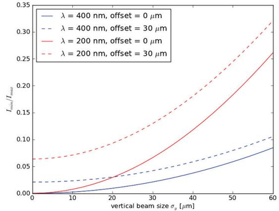
Figure 4: Beam size sensitivity at  $\lambda = 200$  and 400 nm,  $E = 2.1$  GeV and  $a = 1.0$  mm with and without beam jitter.
