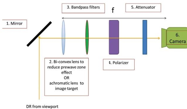
Figure 7: Schematic of optical system.
