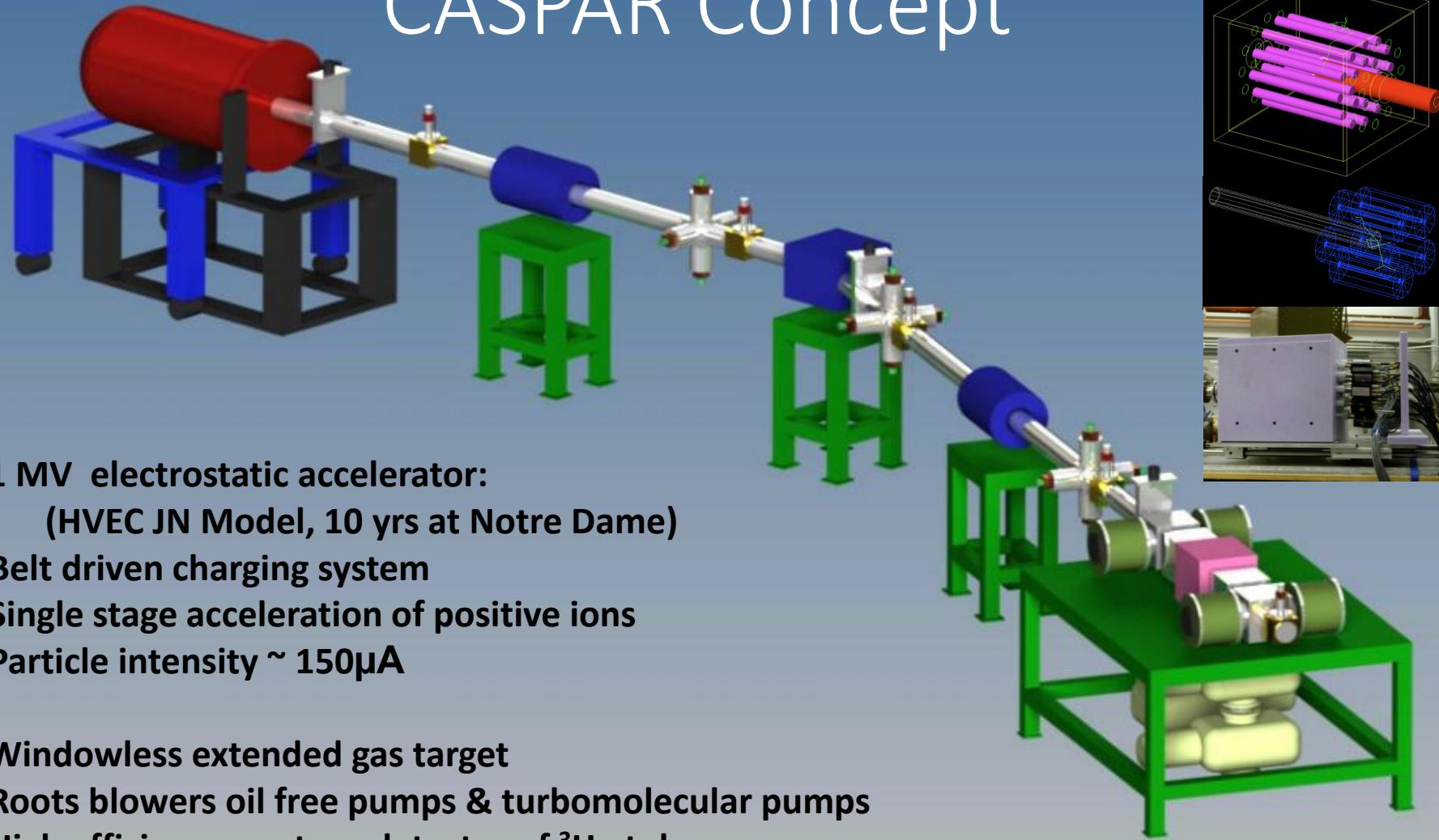
**1 MV electrostatic accelerator:**
