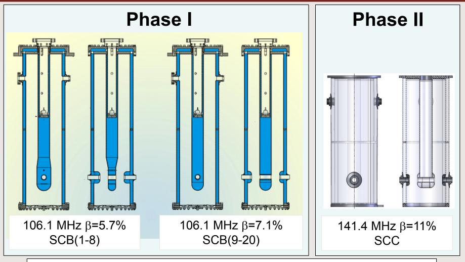
ISAC-II design values:  $V_{eff}$ =1.1MV,  $P_{cav}$ =7W,  $E_p$ =30MV/m,  $H_p$ =60mT
