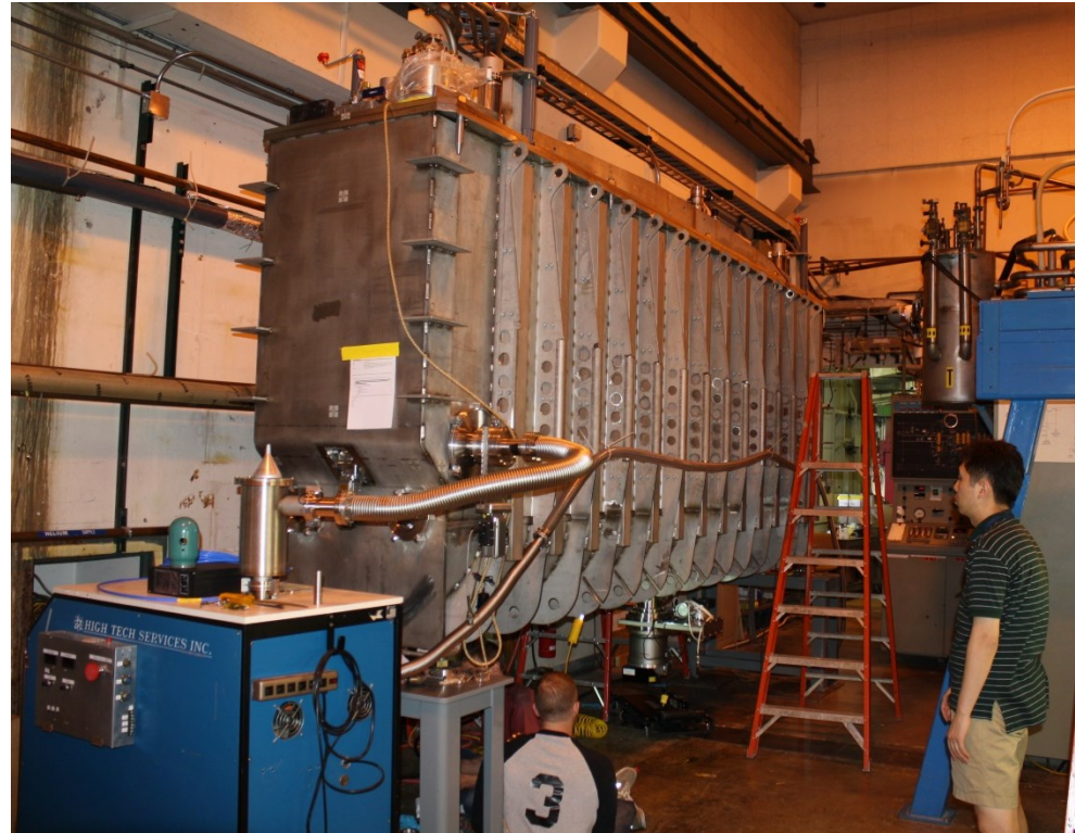
72.75 MHz QWR Cryomodule Leak Testing
