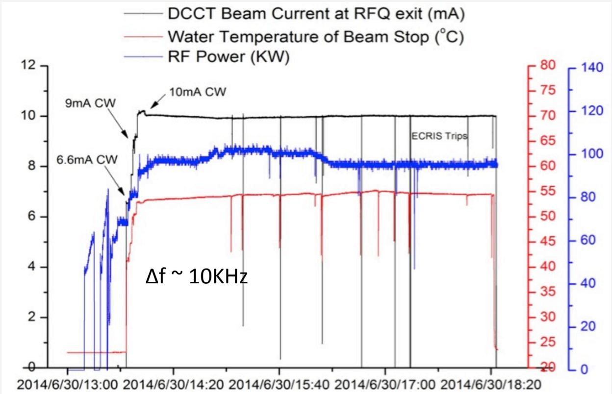
The RF power amplifier is tuned to compensate the beam loading effect.
