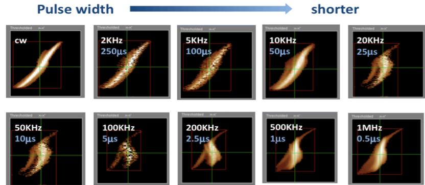
Operation mode transition from pulse mode to CW, beam maybe out of control.
