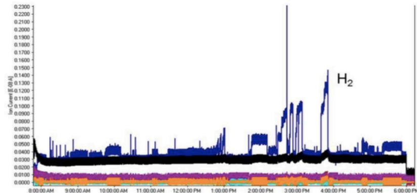
Fig.14. Increase of hydrogen pressure in the MEBT chamber during beam operation
