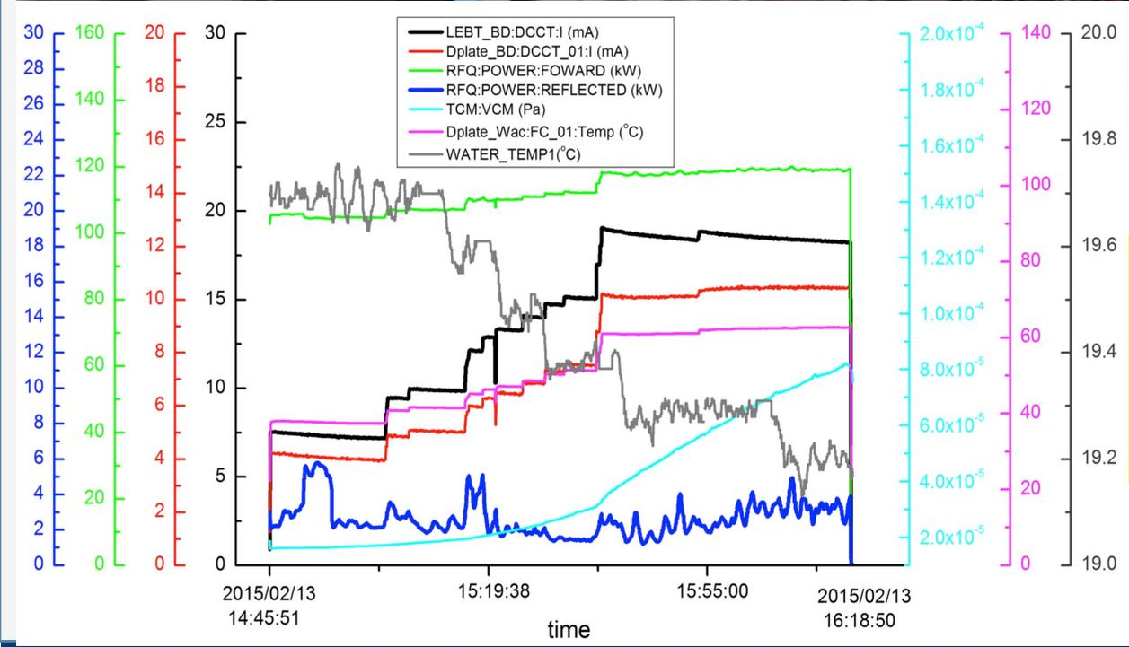
The temperature of RFQ cavity cooling water is tuned manually to decrease the reflection RF power caused by beam loading!
