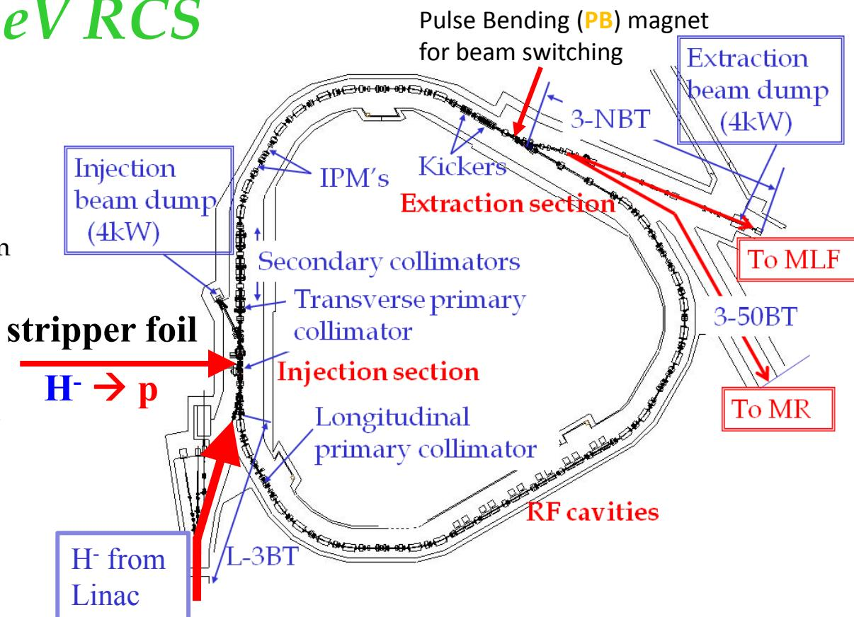
Extracted 3 GeV protons are simultaneously delivered to the neutron and muon production targets in the MLF as well as to the MR for beam injection.
