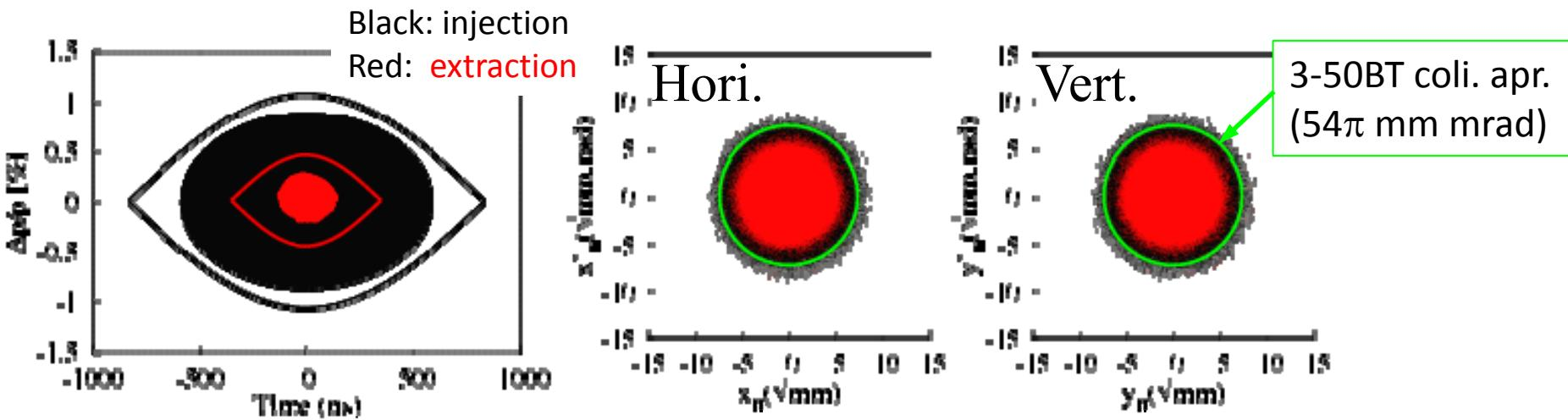
>99.9% transverse emittances of the extracted beam are within 3-50BT collimator aperture.
