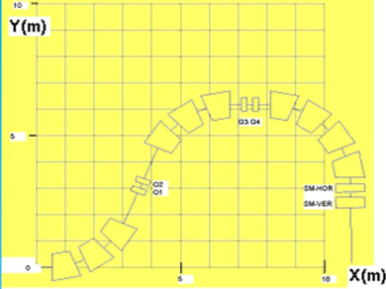
Layout of the JINR superconducting carbon ion gantry.
