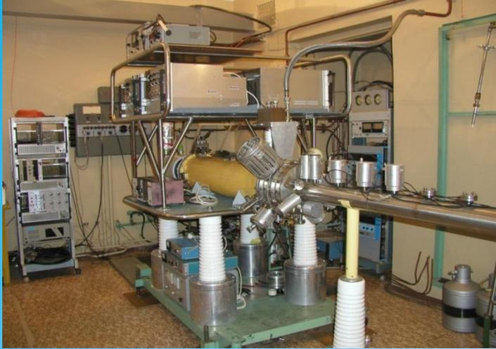
**JINR electron string ion source applied for formation of C<sup>4+</sup> ions**
