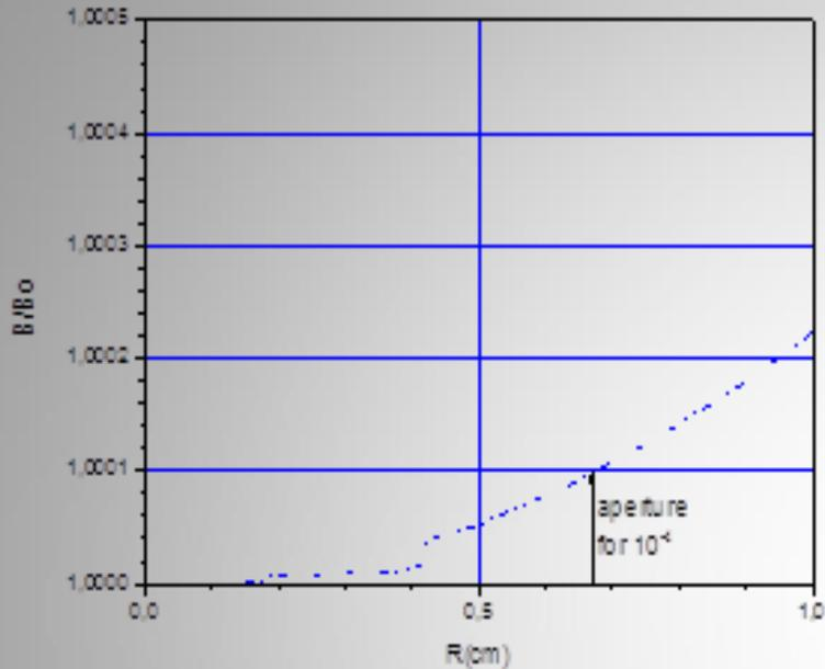
Dependence of magnetic field on transverse coordinate.
