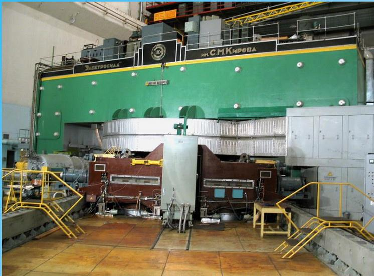
**Synchrocyclotron applied for proton treatment**
