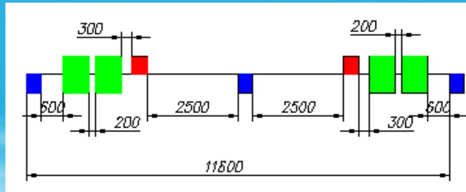
Multiturn injection scheme, orbit and beam envelope: red – injected beam, violet – deflected beam, blue – circulated beam after first injection, green - circulated beam.
