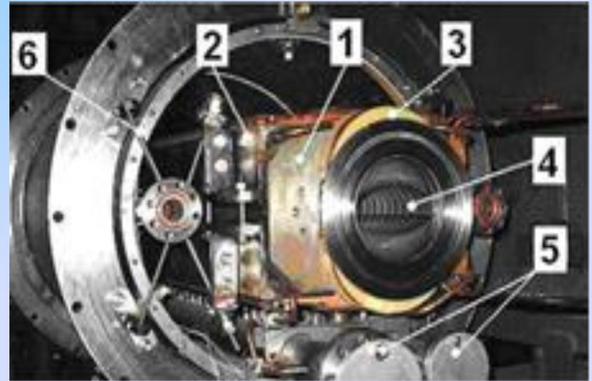
**The Nuclotron type fast cycling 3.6T/s dipole magnets with circulating two phase helium flow in superconducting cable**
