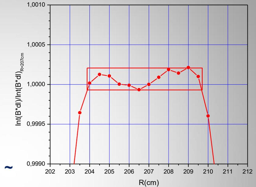
Uniformity of magnetic field integral in the dipole magnet.
