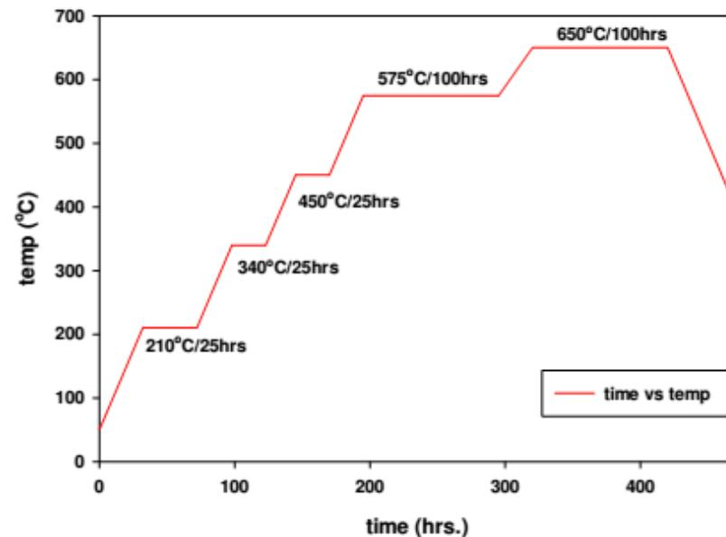
Example heat treatment sequence for ITER wire
