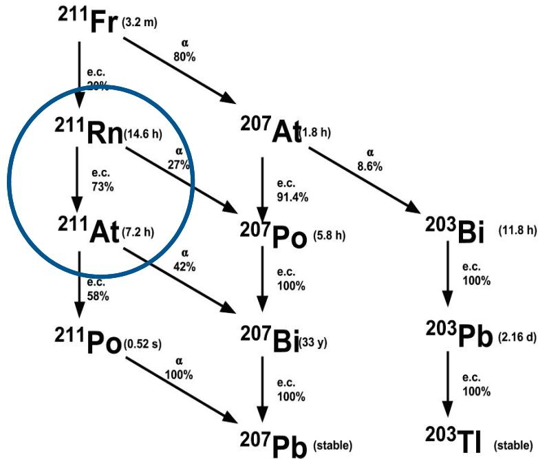
$^{211}\text{Rn}$  was isolated in dodecane, other radioactive inventory was washed away with aqueous solution
