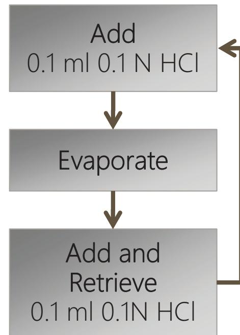
Extraction using 0.1N HCl solution
