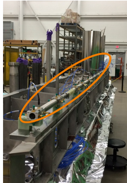
14-sensor wire position monitor installed on ReA6
