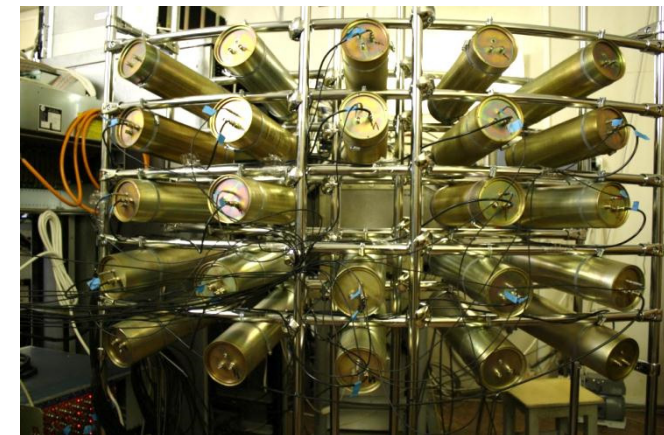
Neutron detector Stylbene crystals scintillator array distance to F5 > 3m TOF accuracy 1%
