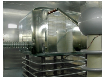
Injector 450 KV 2 sources sputtering
