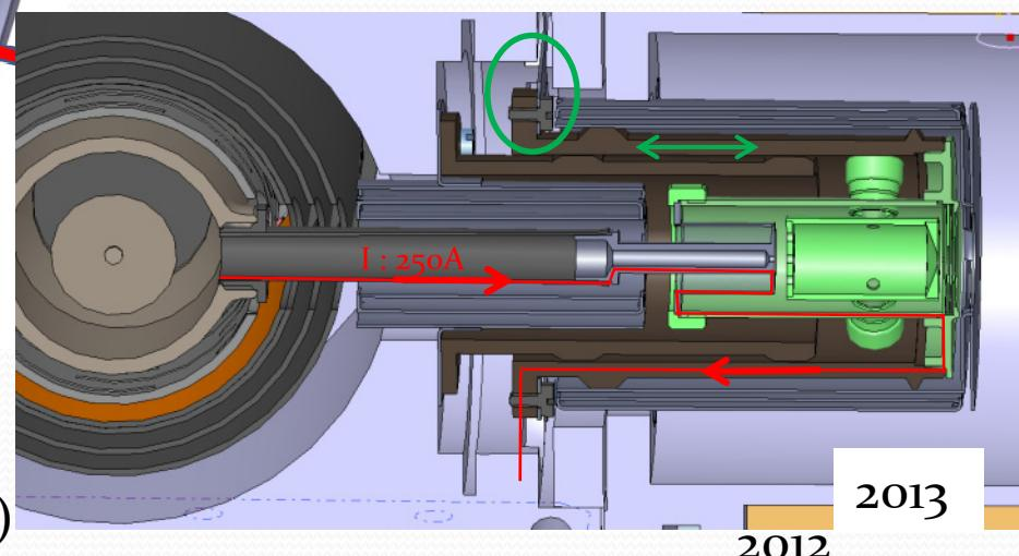
**FEBIAD: Forced Electron Beam Induced Arc Discharge**
