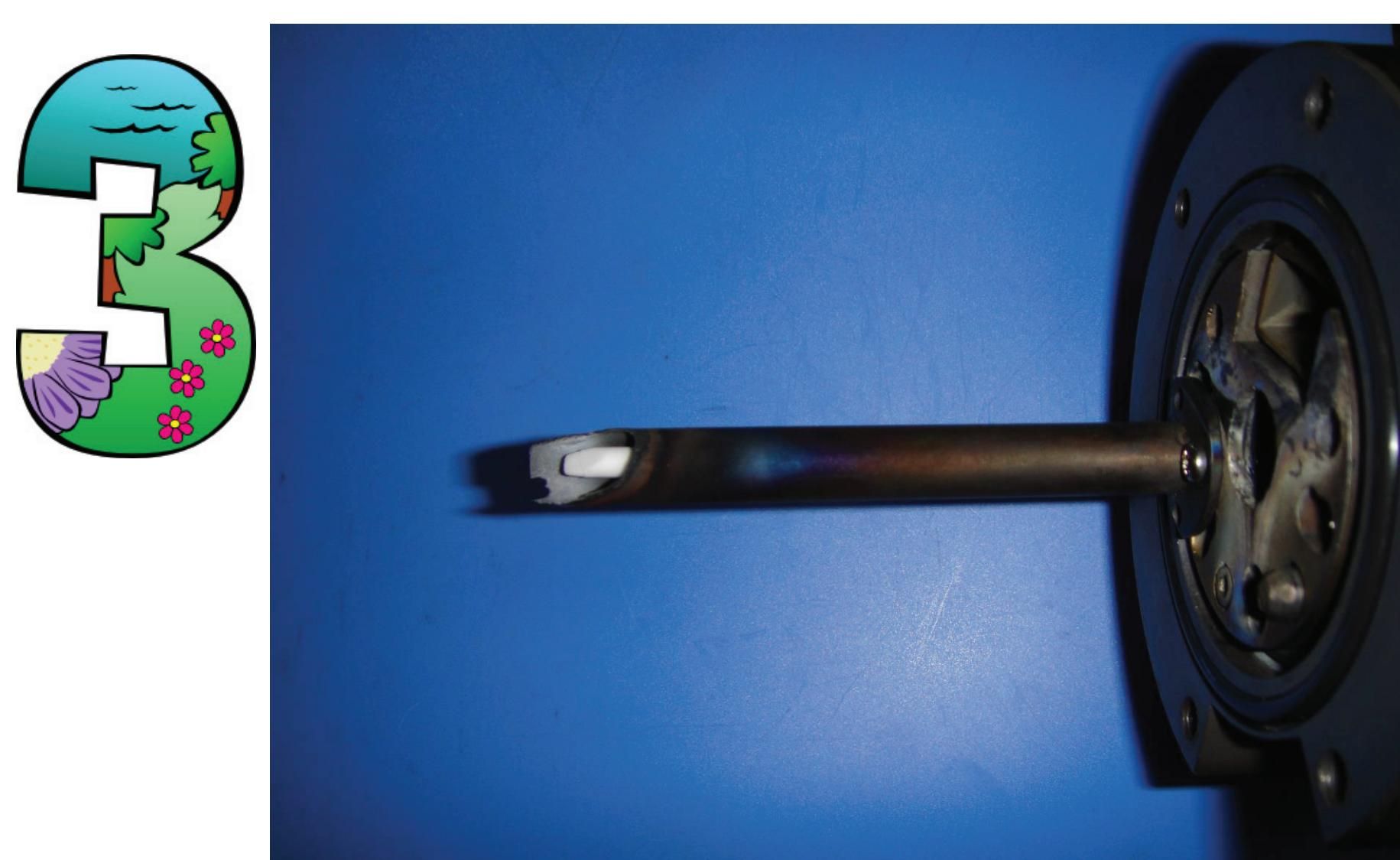
Figure 3: MgO rod with a stainless steel cover.
