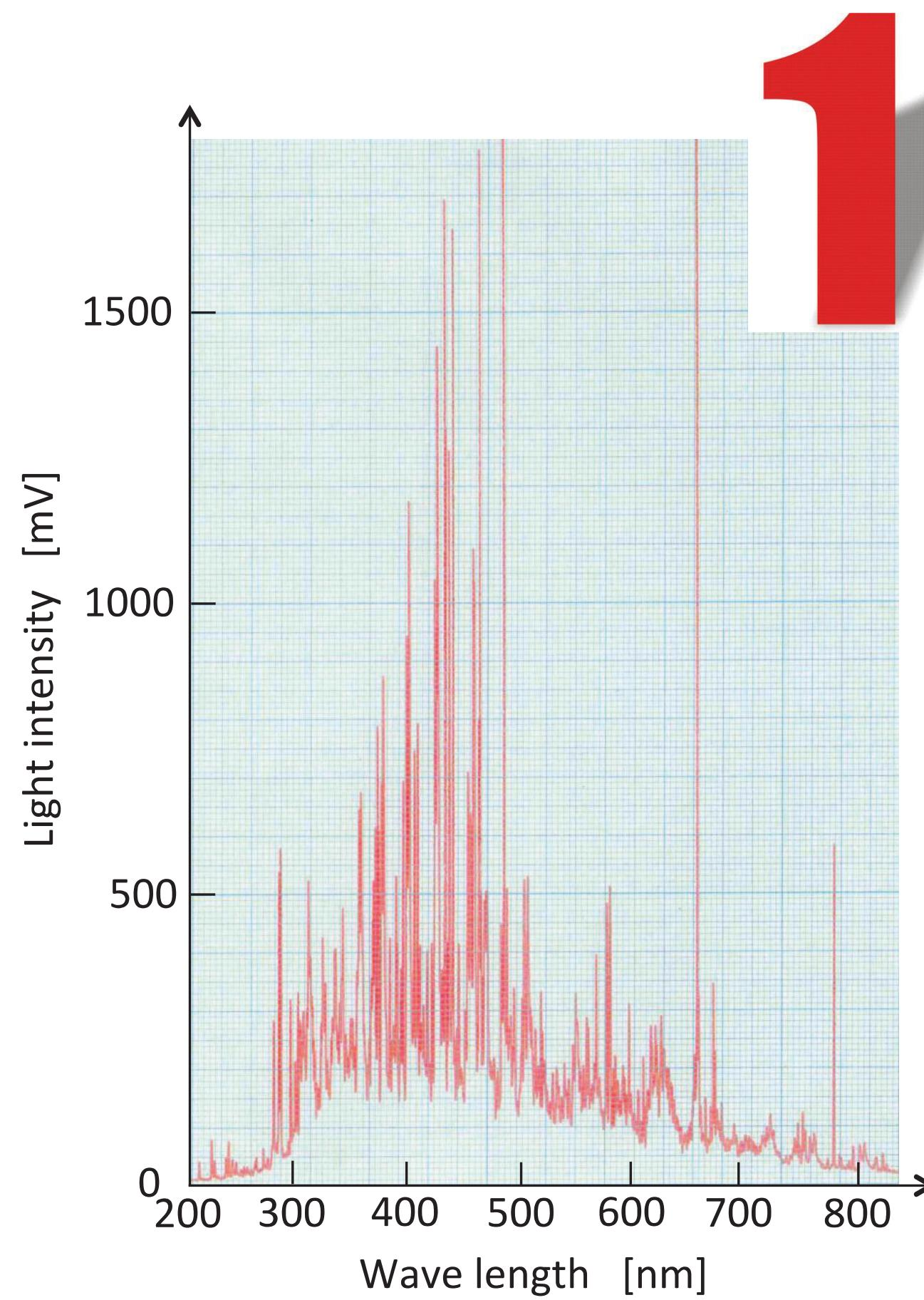
Figure 1: Light intensity spectrum of the residual gas ions after baking for three hours. The peaks of the spectrum are mostly Fe I and Fe II. The pressure and microwave power were  $5.7 \times 10^{-5}\text{ Pa}$  and 100 W, respectively.
