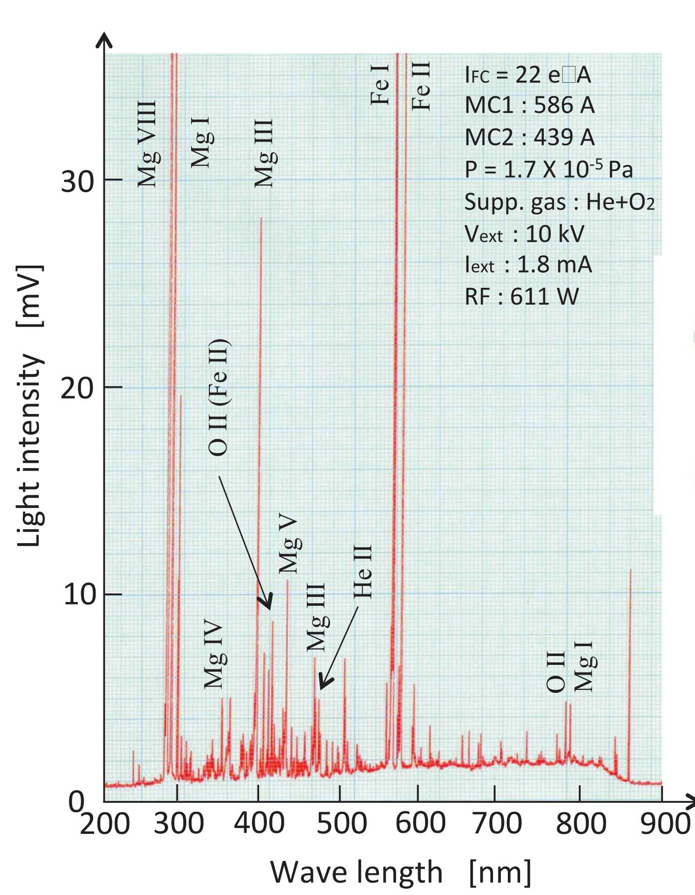
Figure 2: Optical line spectrum during  $^{24}\text{Mg}^{8+}$  ion beam tuning. The shape of the spectrum drastically changed from that of residual gas plasmas. Fe light intensities of residual gas disappeared, and Mg I, III, IV and VIII lines were clearly observed.
