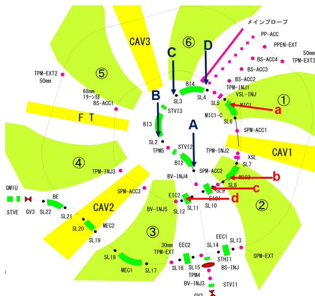
Figure 4: Schematic view of Ring cyclotron: A~D are baffle slits on injection line, a and b are slits of magnetic channel and c and d are electrostatic channel.
