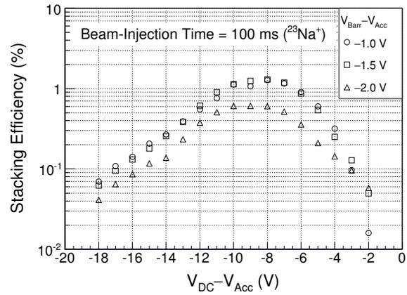
Figure 7: Dependency of the experimental ion stacking efficiency  $\epsilon(t)$  of  $^{23}\text{Na}^+$  on  $V_{\text{Barr}}$  and  $V_{\text{DC}}$  for  $t = 100 \text{ ms}$  where  $V_{\text{RF}} = 210 \text{ V}$ , and  $\omega/2\pi = 1.9 \text{ MHz}$ .
