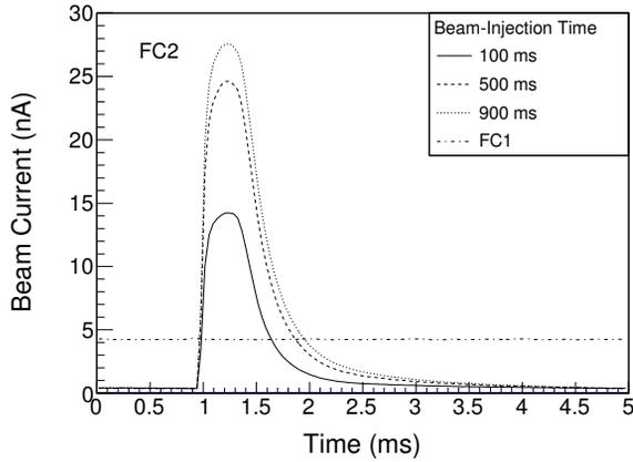
Figure 5: Typical waveforms of the  $^{23}\text{Na}^+$  beam extracted from the buncher observed by FC2 for the beam-injection time of 100 ms, 500 ms and 900 ms where  $V_{\text{Barr}} = V_{\text{acc}} - 1.3 \text{ V}$ ,  $V_{\text{DC}} = V_{\text{acc}} - 6.7 \text{ V}$ ,  $V_{\text{RF}} = 150 \text{ V}$  and  $\omega/2\pi = 1.9 \text{ MHz}$ . The dot-and-dash line shows the waveform of the injected beam observed by FC1.
