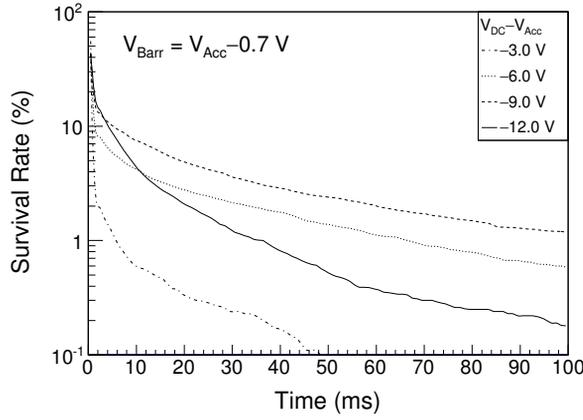
Figure 1: Averaged survival rate  $\langle S \rangle_{\text{RF}}(t)$  of  $^{133}\text{Cs}^+$ . Accelerating voltage of the ions is  $V_{\text{Acc}} = 6.0 \text{ kV}$ , DC voltage applied to the barrier electrodes is  $V_{\text{Barr}} = V_{\text{Acc}} - 0.70 \text{ V}$ , and amplitude and frequency of the RF voltage are  $V_{\text{RF}} = 300 \text{ V}$  and  $\omega/2\pi = 1.6 \text{ MHz}$  respectively.
