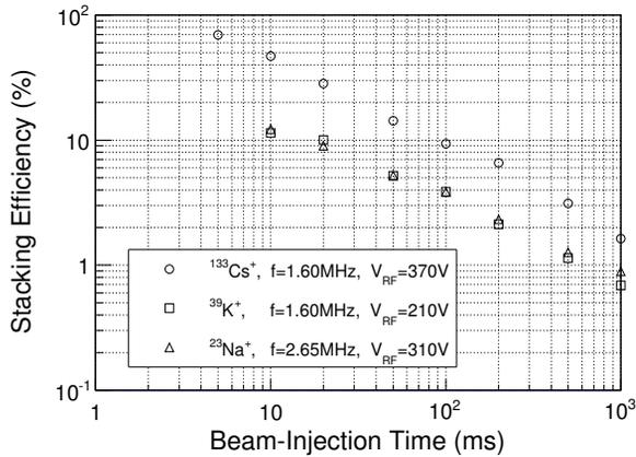
Figure 6: Experimental ion stacking efficiencies  $\epsilon(t)$  of the  $^{133}\text{Cs}^+$ ,  $^{39}\text{K}^+$  and  $^{23}\text{Na}^+$  beams. Values of  $V_{\text{Barr}}$ ,  $V_{\text{DC}}$ ,  $V_{\text{RF}}$  and  $\omega$  have been optimized for each beam.
