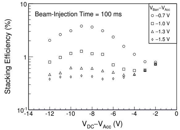
Figure 3: Ion stacking efficiency  $\epsilon(t)$  of  $^{133}\text{Cs}^+$  plotted versus  $V_{\text{DC}} - V_{\text{Acc}}$  for the beam injection time of  $t = 100 \text{ ms}$ .  $V_{\text{Acc}}$ ,  $V_{\text{RF}}$  and  $\omega$  have same values as in Figure 1.
