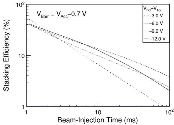
Figure 2: Ion stacking efficiency  $\epsilon(t)$  of  $^{133}\text{Cs}^+$  where  $t$  is the beam injection time.  $V_{\text{Acc}}$ ,  $V_{\text{Barr}}$ ,  $V_{\text{RF}}$ ,  $\omega$  and  $V_{\text{DC}}$  have same values as in Figure 1.
