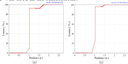
Figure 4: Comparison of the evolution of the beam profile along the LEBT with the slit, (a) shows the H<sub>2</sub><sup>+</sup> ion losses and (b) shows the H<sub>3</sub><sup>+</sup> ion losses.
