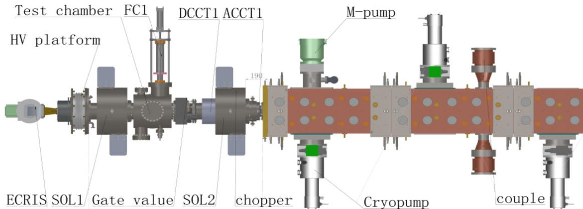
Figure 1: The layout of the ADS LEBT and parts of RFQ.
