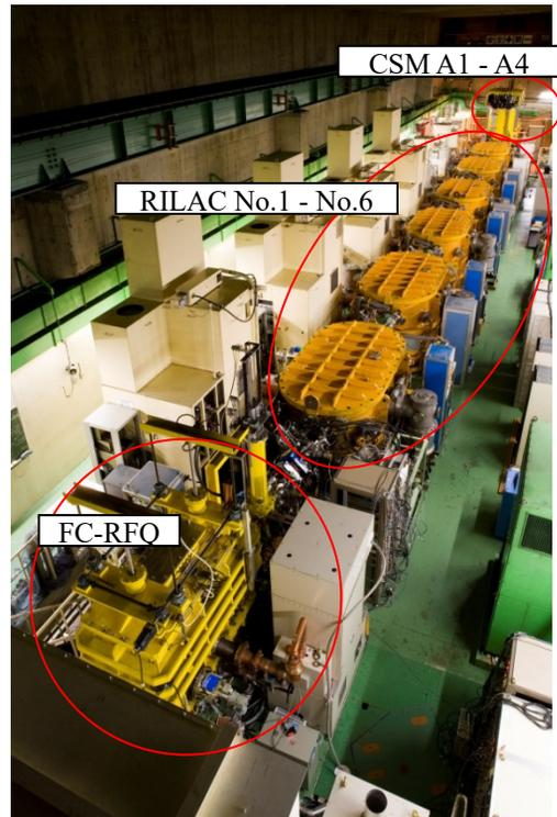
Figure 3: Photograph of FC-RFQ, RILAC, and CSM.
